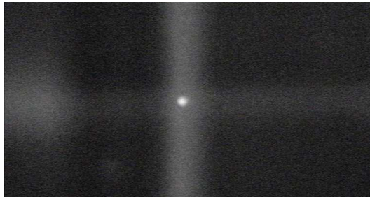
Figure 3.4.: CCD-image of the cloud of cold atoms in the magneto-optical trap (observation direction along the dipole trap axis). The vertical and horizontal lines show light scattered by hot background gas in the cooling beams. At the intersection region a cloud of approximately 3 \times 10^4 cold atoms can be observed (the atom number was estimated from the measured fluorescence).
