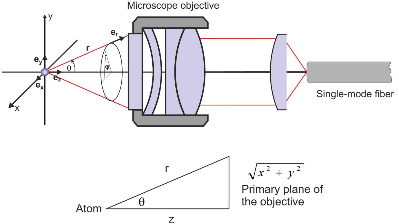
Figure 4.7.: The fluorescence light follows the classical dipole radiation from an atomic dipole arranged along the unit vectors  $e_x$ ,  $e_y$  and  $e_z$ . The  $x$  and  $y$  plane define the plane perpendicular to the optical axis of the objective.[26].
