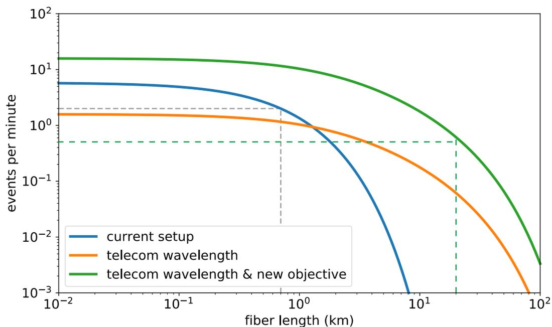
Figure 3.4.: Events per minute for wavelengths 780nm (old objective), 1522nm (old objective) and 1522nm including the new objectives. The gray dashed line shows the current event rate at a distance of 700m. The new objective could more than compensate for the conversion losses to the telecom yielding an estimate of 0.5 remote entanglement events per minute, for a fiber length of 20km shown by the green dashed line.
