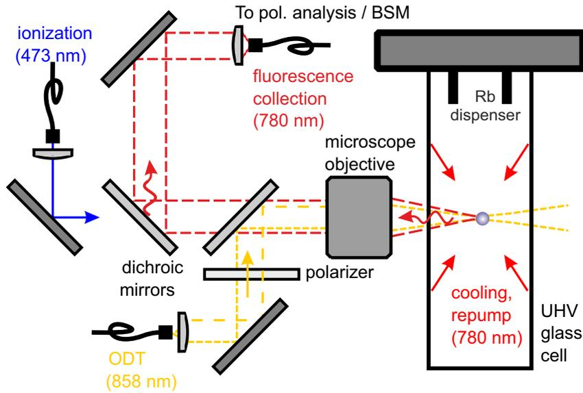
Figure 5.1.: Sketch of the optical setup for the new microscope objective which focusses the dipole trap and the ionization beam to the center of the vacuum glass cell. The fluorescence is collected by the same objective and coupled into a single-mode fiber. The dichroic mirrors separate the three different wavelengths from the optical axis of the objective.
