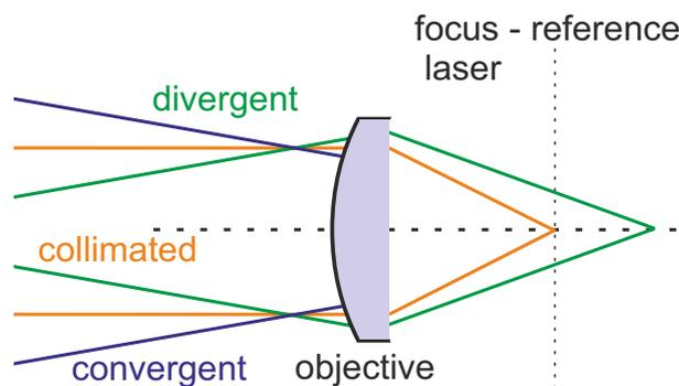
Figure 5.14.: The foci z-position of the three wavelengths may differ due to chromatic aberrations of the objective. This is resolved by adjusting the collimation lenses of the incoming beams depending on the foci displacement.
