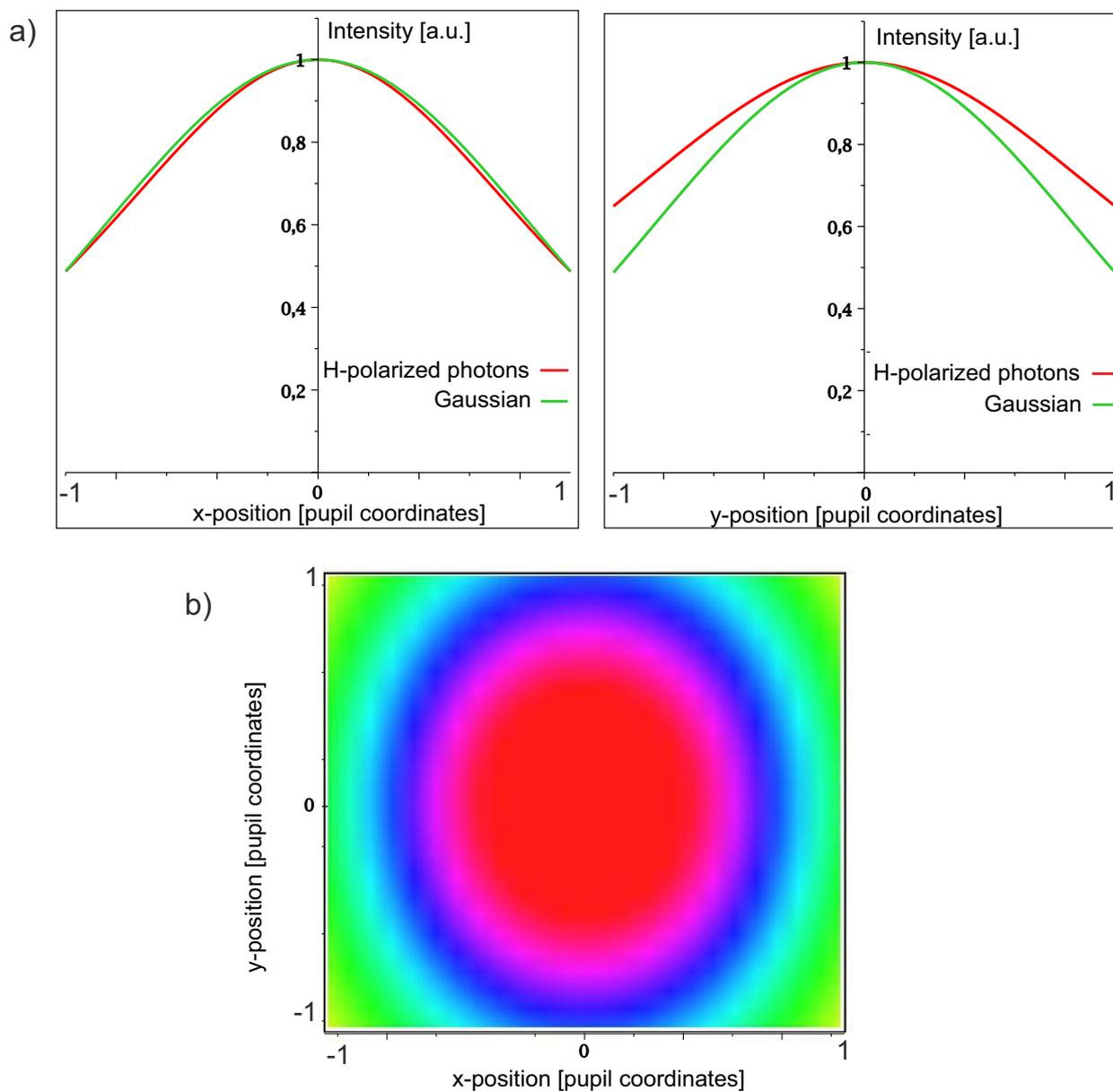
Figure 4.9.: a) Cross section of the H-polarized photon intensity on the primary plane of the objective in x-y direction. The red line depicts the photon intensity and the green line a Gaussian fit with the same parameters for both plots. b) 2D plot of the photon intensity distribution on the primary plane of the objective. The shape for H-polarized photons is an ellipse with a larger extension in y direction.
