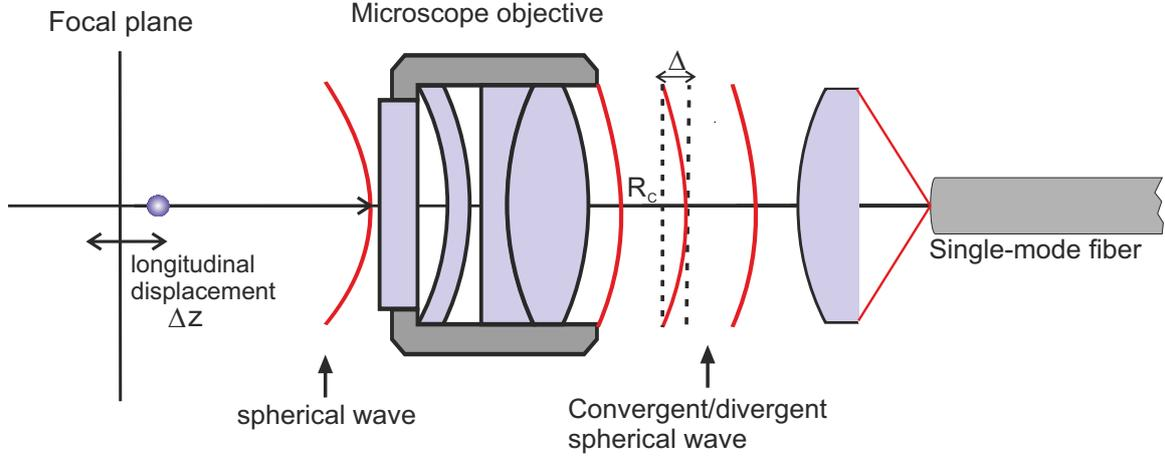
Figure 4.5.: The atom is displaced from the focal plane due to its thermal energy. For longitudinal displacement this leads to a change of curvature of the spherical wave after the objective which reduces the coupling efficiency.
