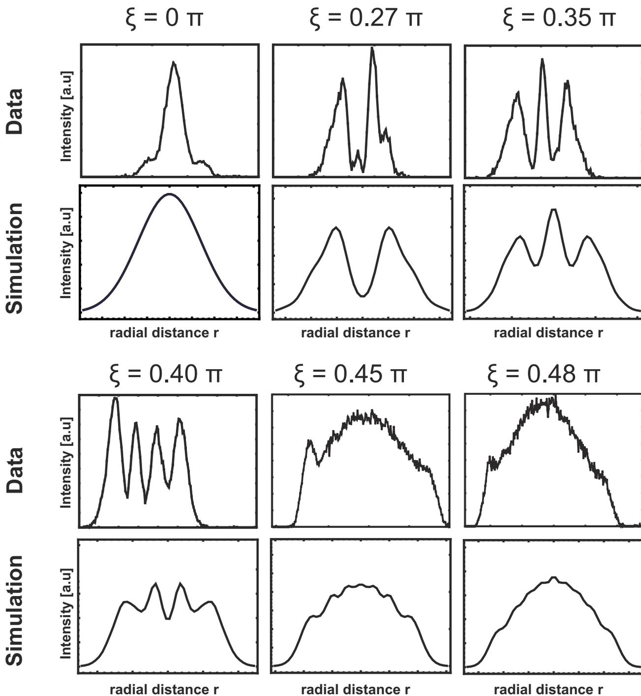
Figure 5.2.: Experimental and simulated intensity profiles for a gaussian beam with spherical aberrations at several positions as a function of the guoy phase. The plotted simulated data is for an  $S$  parameter of 0.7 which yielded the best agreement between measured- and simulated data.
