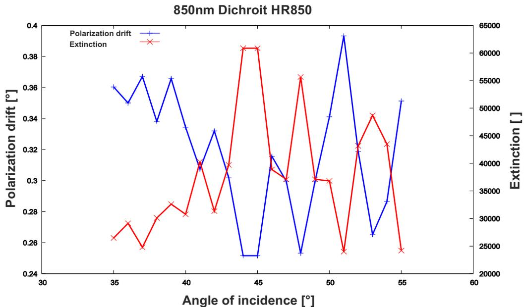
Figure 5.5.: Polarization preservation of the optical dipole trap beam after being reflected by the dichroic mirror for several angles of incidence. The graph shows extinction ratios and the corresponding change in polarization on the Bloch sphere. We get a minimum extinction ratio of  $\frac{1}{25000}$  which is sufficient for the experiment.
