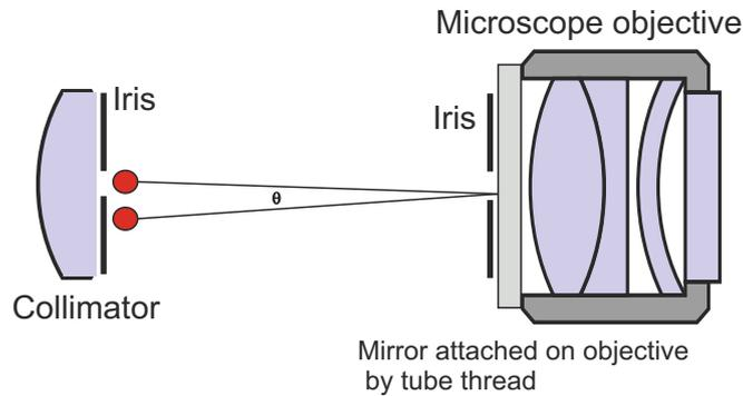
Figure 5.8.: Procedure for the alignment requirement of the incoming beam. Overlap the back reflection of the incoming beam by introducing a mirror in front of the objective.
