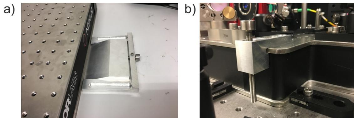
Figure 5.11.: Two options for lifting the breadboard in order to align the glass plate to the objective once the setup is inserted in the main experiment. (a) A wedge lifts the breadboard. (b) Screws on each side lift the breadboard.
