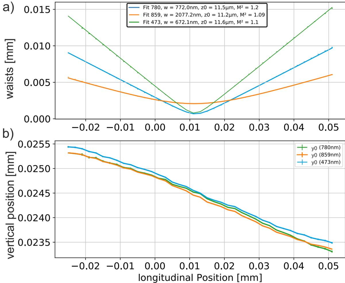
Figure 5.15.: Final focus scan in vertical direction. Plot a)  $M^2$  measurement - Beam radius  $w(z)$  measured for several longitudinal positions for fluorescence collection (blue) dipole trap (orange) and ionization beam (green) with a least square fit to the measured data. The foci are overlapped in  $z$ -direction with an accuracy of 300 nm Plot b) shows the corresponding vertical positions for the respective  $w(z)$ . The three beams are overlapped with an accuracy of 50 nm.
