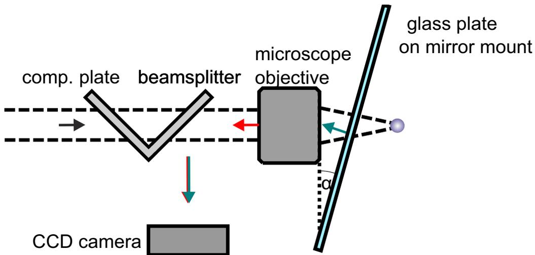
Figure 5.9.: Alignment scheme for the angle between the vacuum glass cell and the objective. By introducing a beamsplitter we overlap the reflections of the objective with the reflections coming from the vacuum glass plate on a CCD camera. The vacuum in the real experiment is mimicked for test purposes by an identical glass plate in terms of coating and thickness.
