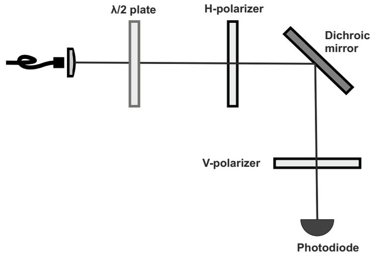
Figure 5.4.: The fraction of H-polarized light coming out of the fiber is maximized by a  $\lambda/2$ -plate. The first H-polarizer fixes the polarization and right after the dichroic mirror a V-polarizer to test the change of polarization by measuring the remaining intensity on a photodiode. The preservation was measured for several angles of the dichroic mirror.
