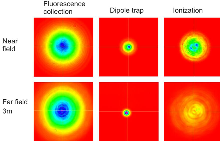
Figure 5.17.: Beam profile of the three beams before the objective in the near (0.5m) and far field (3m). The cross determines the center of mass of the intensity distribution of the fluorescence collection. It can be seen, that for the overlapped case, the relative position of the two remaining beams is slightly displaced. This gives an indication for future alignment verification.
