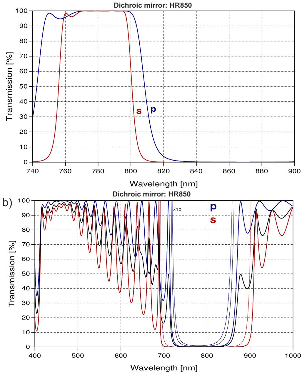
Figure 5.3.: a) Transmission of the s- and p-polarization on the dichroic that is high reflective for the dipole trap laser and high transmissive for the fluorescence collection. b) Transmission of the s- and p-polarization on the dichroic that is high reflective for the fluorescence collection and high transmissive for the ionization laser. In all cases, an equal transmission of s- and p-polarization is given with at least 99.9%.
