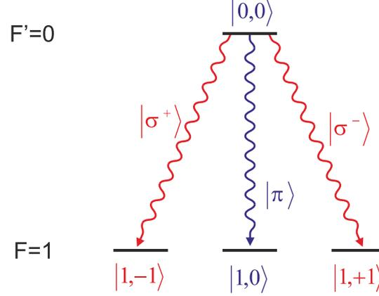
Figure 2.2.: Atom-photon entanglement scheme. Spontaneous decay of the excited state  $5^2P_{3/2} |F' = 0, m_{F'} = 0\rangle$  via either emitting a  $|\sigma^+\rangle$  or  $|\sigma^-\rangle$  polarized photon. The  $\pi$  polarized light to the  $|F = 1, m_{F'} = 0\rangle$  state is automatically filtered out due to the orientation of the quantization axes[26].
