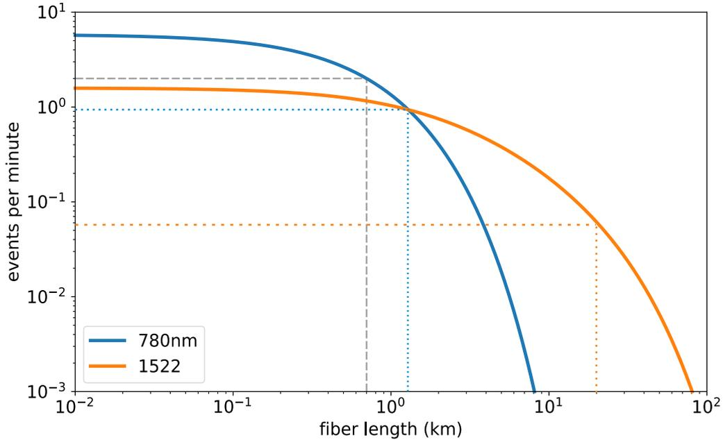
Figure 3.3.: Events per minute at wavelengths 780nm and 1522nm. The grey dashed line shows the current event rate at a distance of 700m. The blue dotted line shows the point from which the conversion to 1522nm pays off (40% photon conversion efficiency, 80% photon detection efficiency) which is after 1.5km. At a fiber length of 20km with photons in the telecom band one obtains  $\simeq 0.06$  events per minute which is marked by the orange line.
