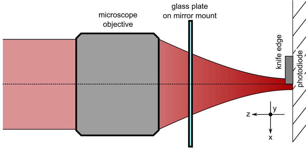
Figure 5.6.: Knife-edge method for measuring the foci after the objective. As a sharp edge we use a gold structure which is placed on a photodiode. The gold-structure is translated through the beam while the photodiode records the resulting intensity profile. From that we can reconstruct the Gaussian focus.
