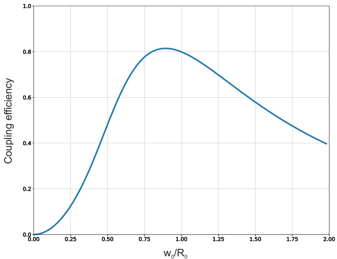
Figure 4.2.: Coupling efficiency of a Gaussian beam with top hat shaped aperture of the objective as a function of the waist of the beam and the objective pupil radius. The maximal coupling efficiency is 81.45% with a optimal waist to objective pupil ratio of 89.3%.
