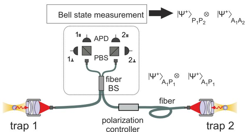
Figure 2.5.: Sketch of the atom-atom entanglement scheme. The basic principle is to create atom-photon entanglement in two separate traps, followed by a coincidental Bell state measurement (Coincident detection of two photons). This leads according to the entanglement swapping protocol to atom-atom entanglement without any direct interaction.
