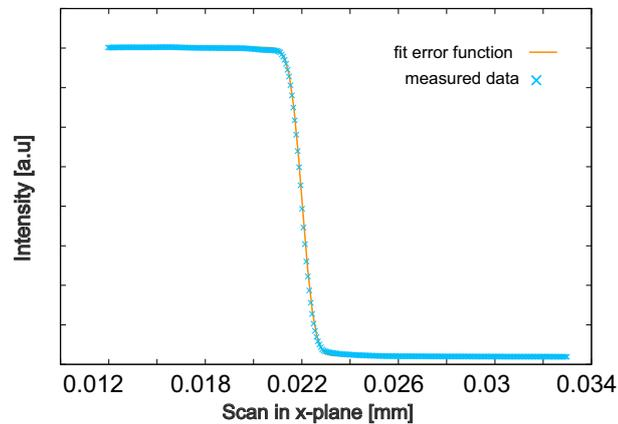
Figure 5.13.: Focus measurement after adjust the glass plate and the incoming beam. The focus has a Gaussian like shape and no smearing artifacts are visible. From that result we conclude that the alignment requirements are met.
