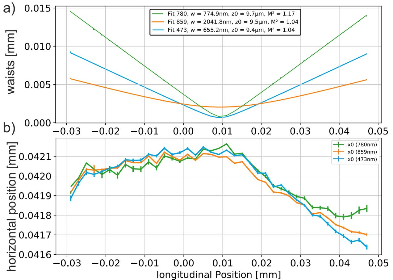
Figure 5.16.: Final focus scan in horizontal direction. Plot a)  $M^2$  measurement - Beam radius  $w(z)$  measured for several longitudinal positions for fluorescence collection (blue) dipole trap (orange) and ionization beam (green) with a least square fit to the measured data. The foci are overlapped in  $z$ -direction with an accuracy of 300 nm Plot b) shows the corresponding horizontal positions for the respective  $w(z)$ . The three beams are overlapped with an accuracy of 50 nm.
