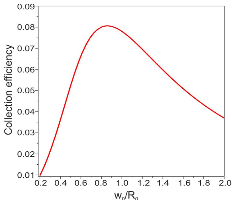
Figure 4.10.: Photon collection efficiency for the atomic dipole emitting H-polarized photons. The maximal collection efficiency is 8.07% with an optimal ratio of the waist  $w_0$  of the collimator and the objective pupil radius  $R_0$  of 85.44%.
