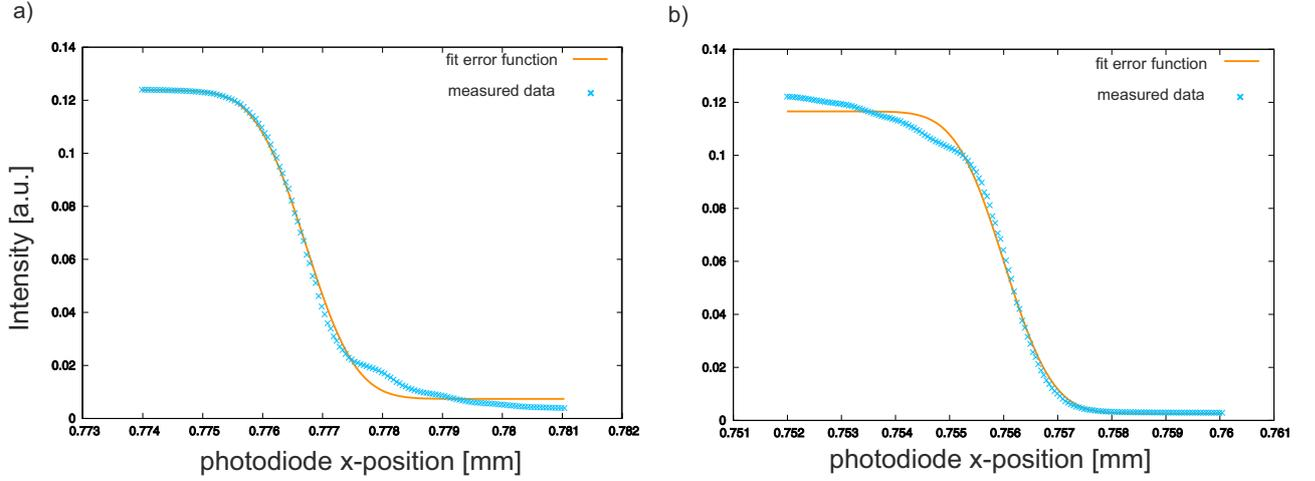
Figure 5.12.: Plots for the measured intensity as a function of the position on the photodiode in the focal plane. (a) The glass plate is tilted towards the objective which induces smearing at the edges of the focus (b) The glass plate is tilted in the opposite direction as in (a). The smearing happens then on the opposite side of the focus.
