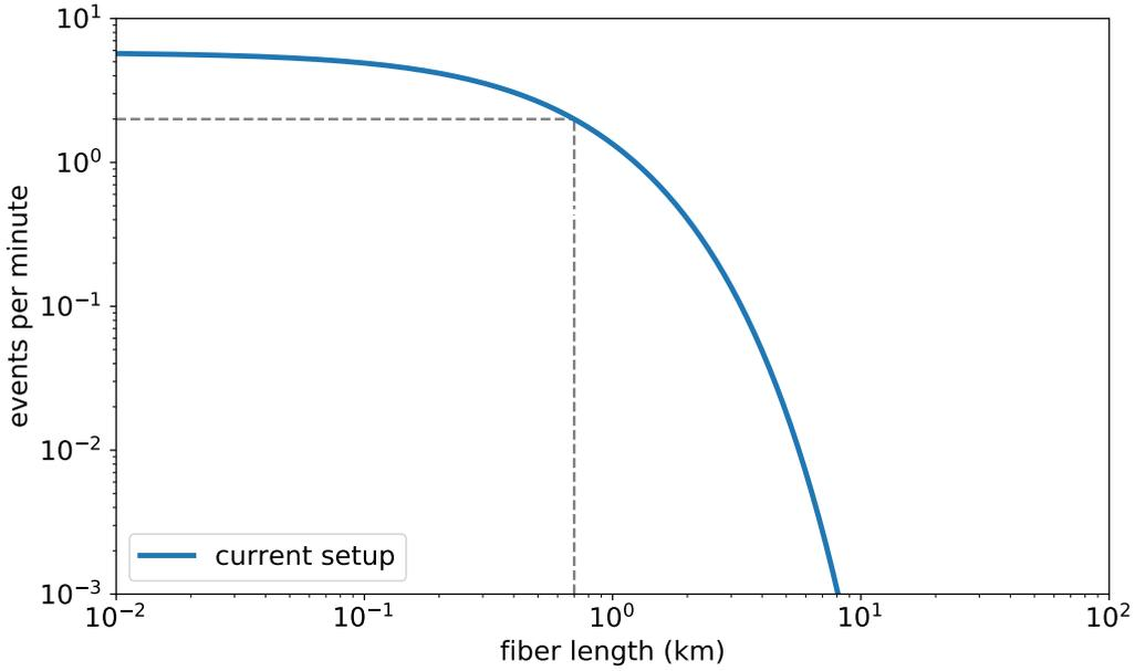
Figure 3.2.: Events per minute for the current setup with a photon wavelength of 780nm. The gray line shows the current length of the optical fiber with 700m which yields around 2 atom-atom entanglement events per minute.
