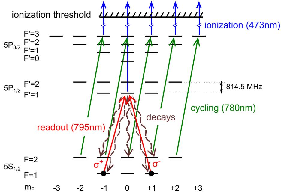
Figure 2.4.: Atomic state readout scheme. The polarization of the readout laser determines whether the atomic state gets excited and subsequently ionized. This process is called Zeeman state selective ionization. Additionally, the cycling laser re-excites atoms which decayed before the ionization [19].
