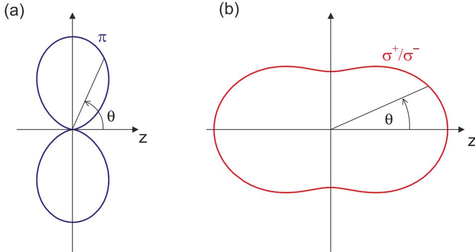
Figure 2.3.: Dipole emission characteristics of a)  $\pi$ - and b)  $\sigma^\pm$ -polarized light. The emission intensity is dependent on the angle  $\theta$  relative to the quantization axis. There is no emission of  $\pi$ -polarized light in  $z$ -direction whereas  $\sigma^\pm$ -polarized emission in this direction is maximal [26].
