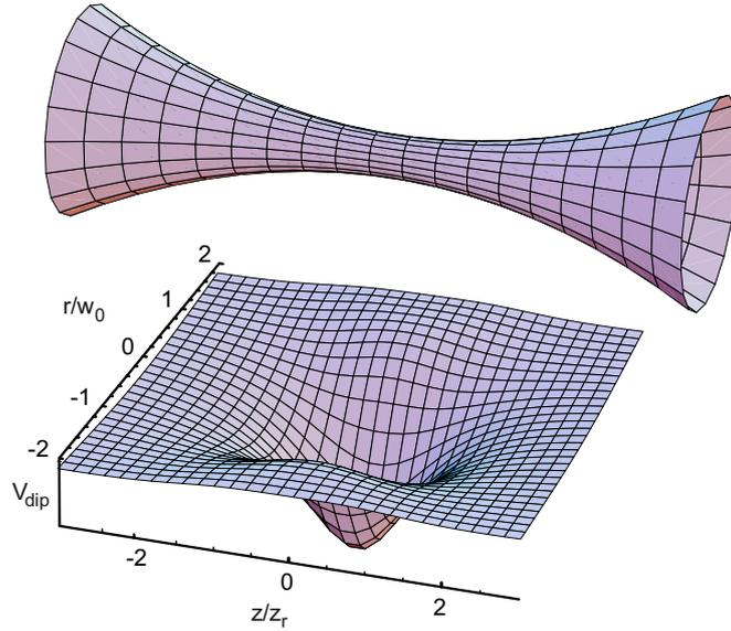
Figure 2.1.: Schematic drawing of a focussed  $TEM_{00}$  gaussian beam and the corresponding trapping potential [27].
