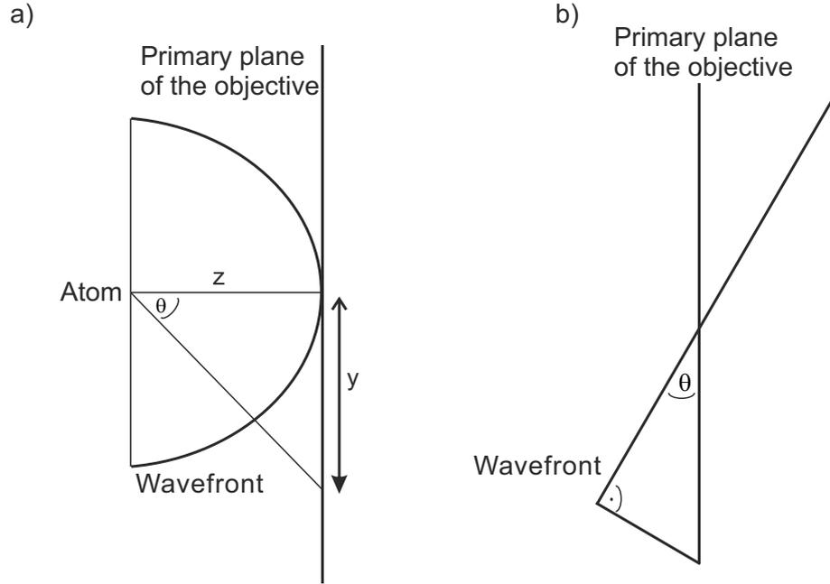
Figure 4.8.: (a) The spherical projection describes the conversion from an angle element of a sphere onto a surface element in a plane. (b) Derivation of the scaling factor by considering an infinitesimal small part of the intersection, where the spherical wave can be approximated plane.
