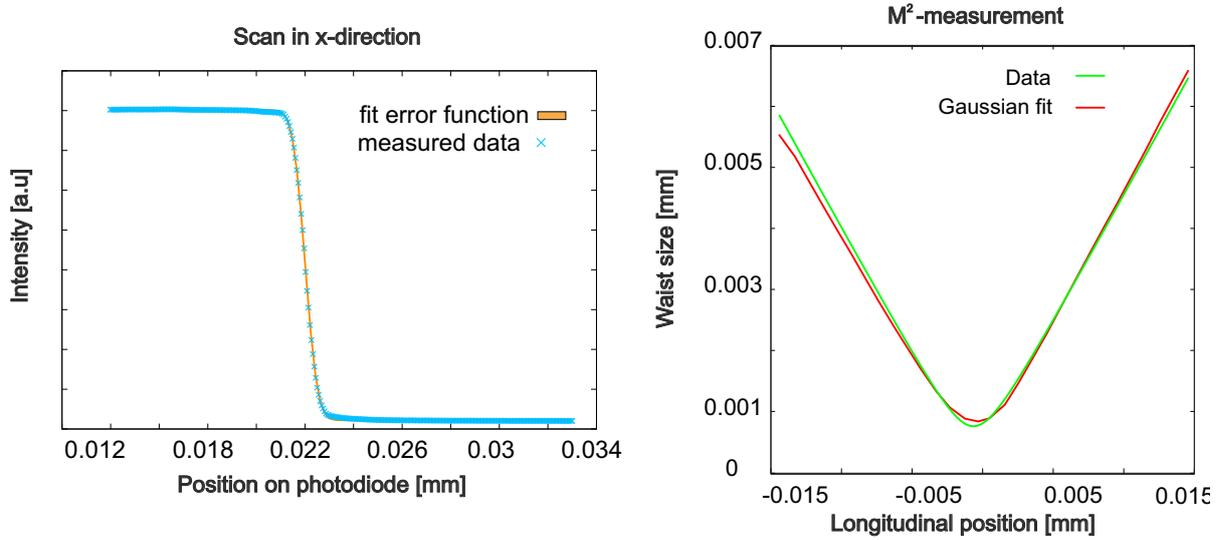
Figure 5.7.: Left) Knife-edge scan in x-direction. Right)  $M^2$  measurement: repetition of a scan in x-direction for several focal position  $z$ .
