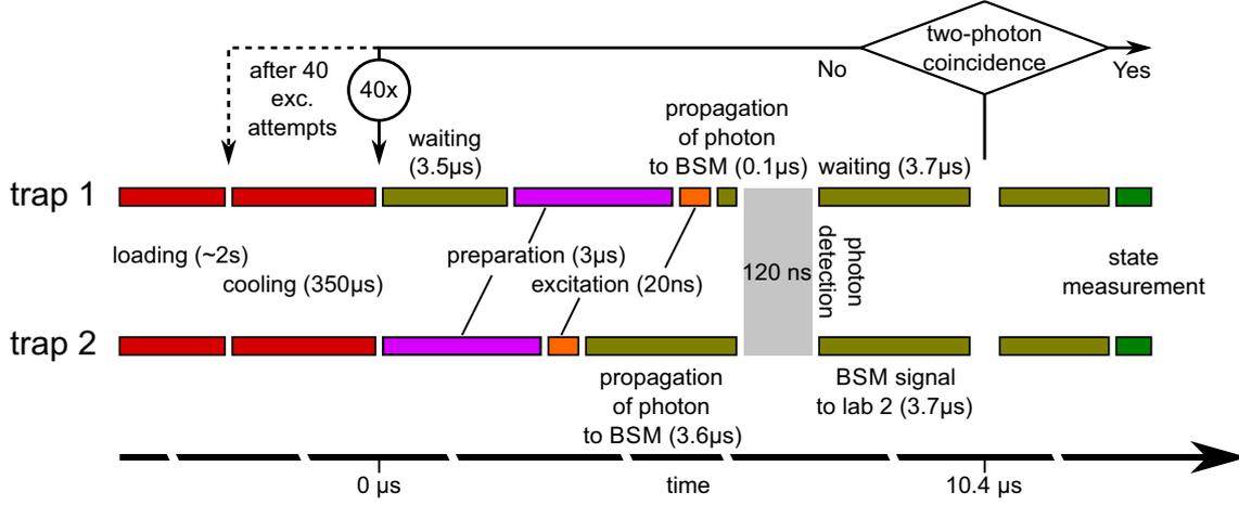
Figure 3.1.: Experimental sequence and timings to entangle two Rubidium atoms in two separate traps. Once there are two atoms loaded in both dipole traps, the previously described pumping and excitation scheme is repeated until successful atom-photon entanglement in both traps is achieved. Each excitation cycle will heat the atom hence there will be a cooling period after 40 excitation repetitions [7].
