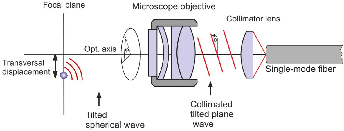
Figure 4.3.: The atom is displaced from the optical axis due to its thermal energy. For radial displacement this leads to a transversal tilt of the emitted plane which reduces the coupling efficiency.
