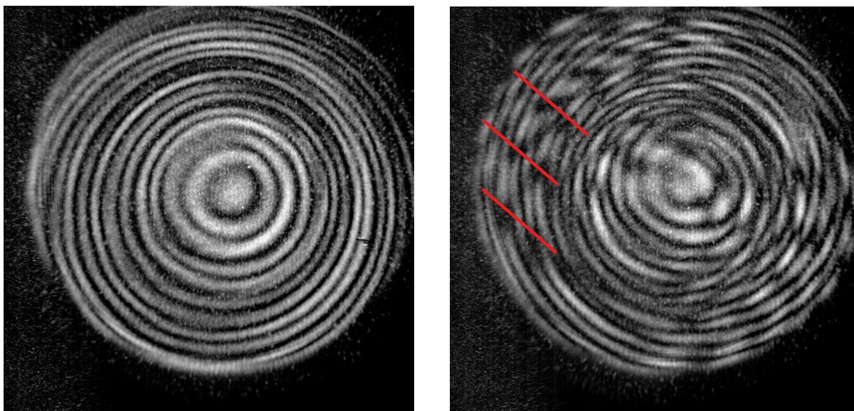
Figure 5.10.: Interference pattern for the overlapped back reflections coming from the objective and the glass plate. The left picture shows only the concentric ring structure which is independent of the orientation of the glass plate. The right side shows additional diagonal interference fringes coming from the interference of objective and glass plate back reflection.
