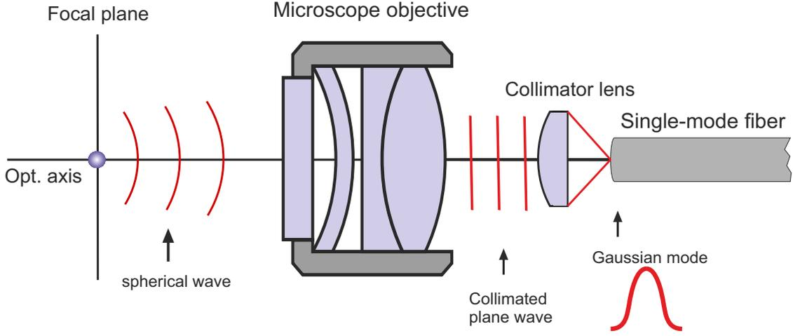
Figure 4.1.: The atom is at the axis of the objective and in the focal plane. The emission of the atom is approximated as a point source. The spherical waves get then converted by the objective into a collimated plane wave and coupled into a single-mode fiber.
