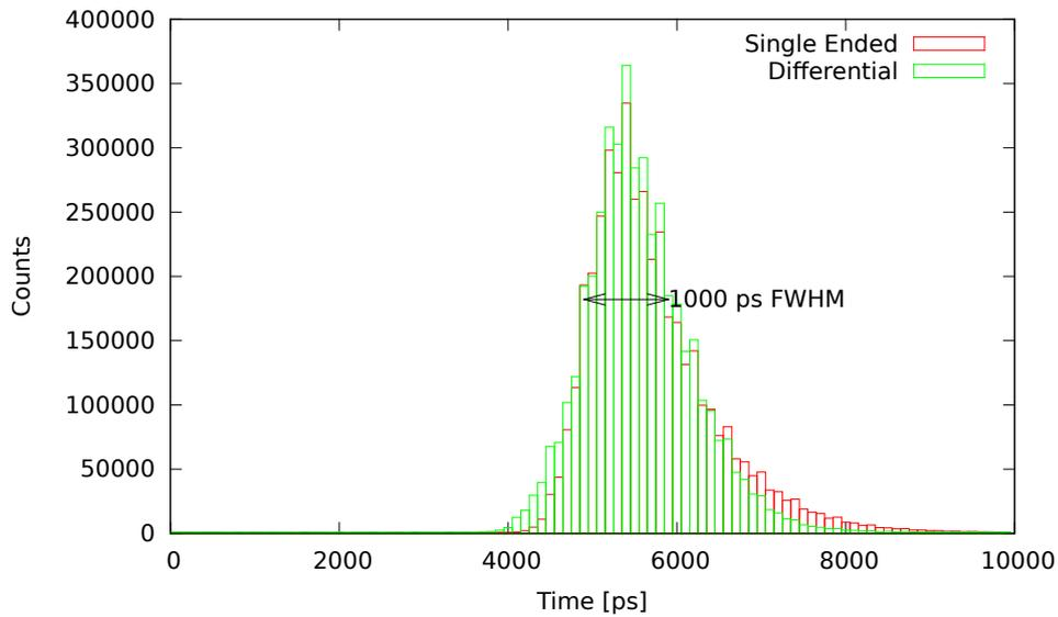
Figure 5.10: The arrival times for a single ended and a differentially connected VCSEL driven with the ONET4291VA.
