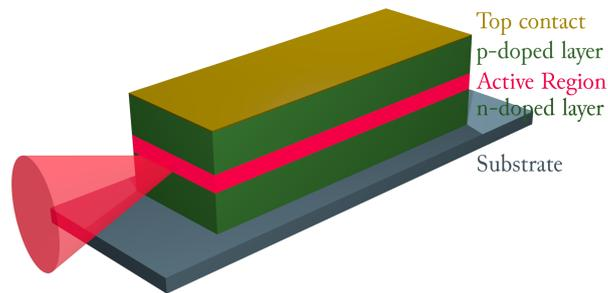
Figure 4.1: Structure of an EEL. The active region is located between two epitaxial layers. Light is emitted through the edge of the active region. The whole structure is placed on a substrate and a top contact is used to inject currents to the EEL. Picture analog to [37] p. 23.
