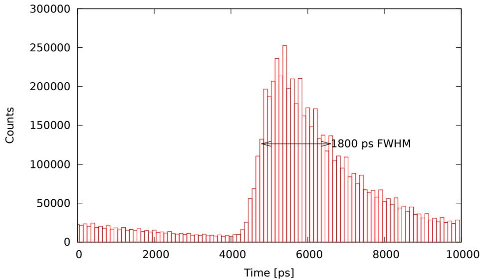
Figure 5.8: Arrival times for photons in a pulse produced with the ONET8501V.
