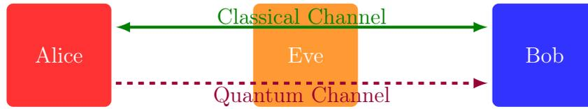
Figure 2.1: Scenario typical to modern communication. Alice and Bob share a classical communication channel on which, however, eavesdropping cannot be prevented. In the QKD scenario an additional quantum channel is added to transmit quantum states from Alice to Bob.
