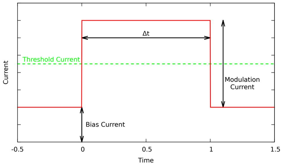
Figure 5.1: The current pulse applied to a VCSEL, with the time and current in arbitrary units. To achieve a high contrast between the on and off state of the diode, one has to ensure, that the bias current lies well below the threshold current and together with the modulation currents exceeds the threshold.
