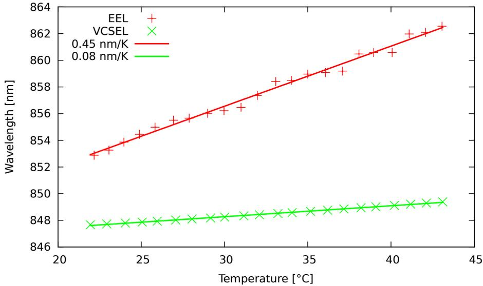
Figure 4.3: The temperature dependence of the spectrum of a VCSEL and an EEL compared. It can be seen that the temperature dependence of VCSELs is much weaker. The solid lines represent linear fits to the measured data, where slopes of 0.45 nm/K and 0.08 nm/K were found, respectively.
