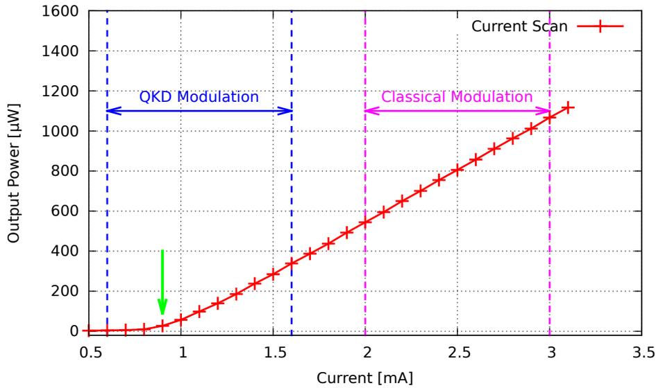
Figure 5.2: The difference between the modulations in quantum and classical communication. In the QKD application it is necessary to modulate the current over the threshold to achieve high contrasts. In classical communication, however, one can afford to modulate the current in the lasing regime, only. The threshold current is marked by the green arrow.
