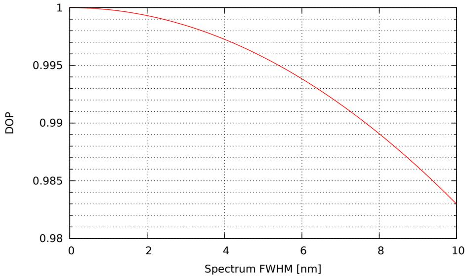
Figure 3.7: The calculated DOP of light at the output of the laser written waveguide. It is shown that the DOP decreases with the FWHM of the spectral distribution of a light source.
