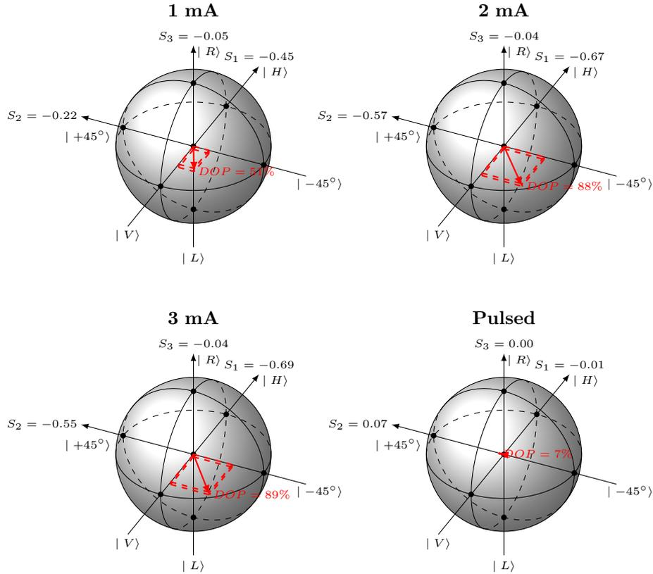
Figure 4.7: The results of the DOP measurements at different currents and during pulsed operation. The normalized values  $S_i/S_0$  for the Stokes parameters are given at the respective axes.
