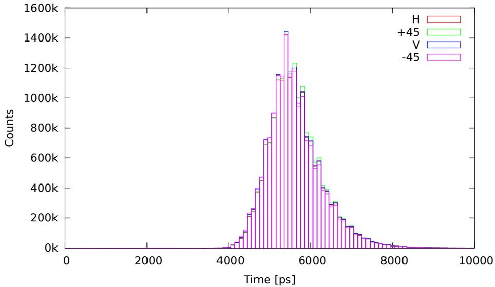
Figure 4.8: The pulses of one VCSEL, time resolved for the projections on the four different polarizations in the equatorial plane of the Poincaré sphere.
