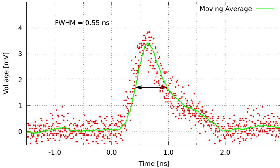
Figure 5.17: The voltage signal of a fast photodiode, while short pulses from one VCSEL were applied. The green curve is a moving average of the data points and yields a FWHM of 550 ps. The red points represent the samples measured on the DSO of 10 consecutive pulses.
