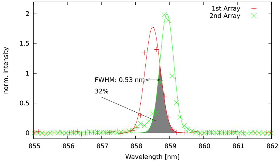
Figure 4.4: The measured spectrum and best-fit curves of two VCSELs from two different VCSEL arrays. The gray area shows the overlap between the two fitted curves of 32%. The curves and the data points are normalized.
