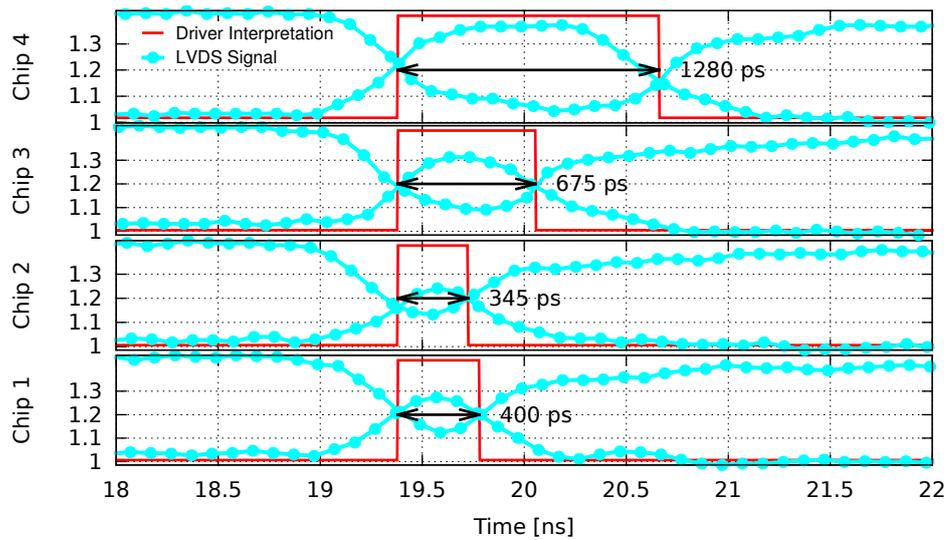
Figure 5.14: The differential signals for the pulses produced by the FPGA. The logical interpretation of those signals is denoted in red for every driver. The respective pulse widths vary due to different propagation delays for the LUTs in the FPGA. The y-axes show the voltage for the two differential lines according to the LVDS standard. All of those signals were individually triggered on a DSO.
