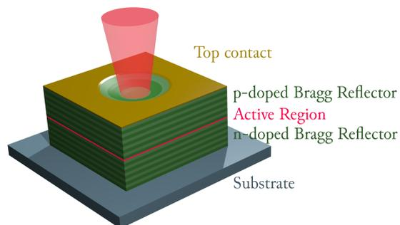
Figure 4.2: The active region of a VCSEL is positioned between p- and n-doped Bragg reflectors, which serve as a cavity. This structure is grown epitaxially, by adding layers of different semiconductors with high and low IOR. Picture analog to [37] p. 23.
