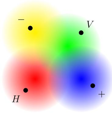
Figure 2.4: Illustration of only partially overlapped beams from four different laser diodes. The dots depict points where Eve can surely distinguish between the four settings, without measuring the polarization. The four different modes from the laser diodes are colored for better understanding.
