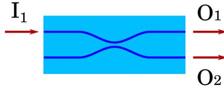
Figure 3.8: Definition of the in and outputs for the directional coupler. With the previous setup, light was coupled into one of the two inputs of an integrated BS  $I_i$ . The “transmitted” output is named  $O_1$  and the “reflected” output is named  $O_2$ .
