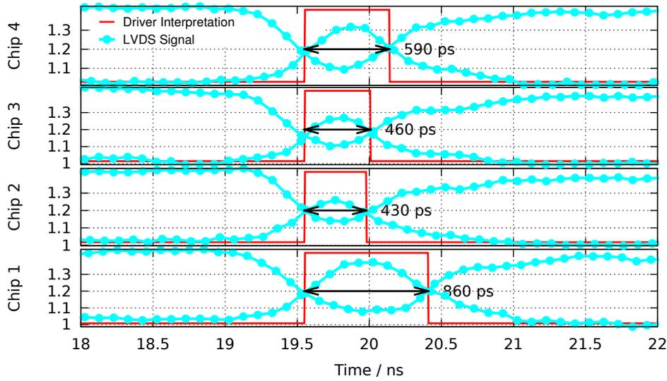
Figure 5.15: The differential signals for pulses after inserting additional logical elements. The difference between the pulse widths has improved, yet is still not sufficient for a secure QKD device. All of those signals were individually triggered on a DSO.
