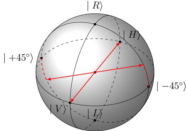
Figure 3.11: The four states sufficient for a QKD. The  $\pm 45^\circ$  polarizations are rotated due to birefringence, yet they are orthogonal to the  $H - V$  axis.
