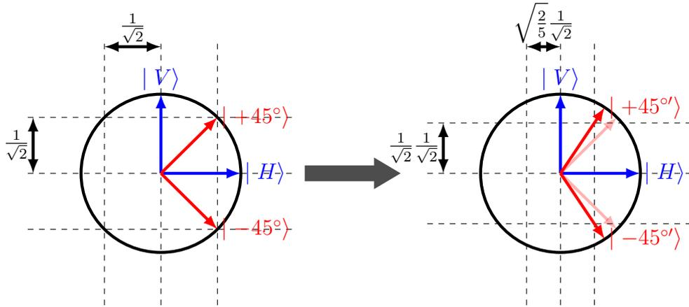
Figure 3.10: Change of the  $\pm 45^\circ$  polarization due to different splitting ratios for  $H$  and  $V$  polarization. The resulting polarizations  $|\pm 45'^\circ\rangle$  are modified towards  $|V\rangle$  in  $O_2$ , because the horizontal polarization gets weaker relative to  $|V\rangle$ .
