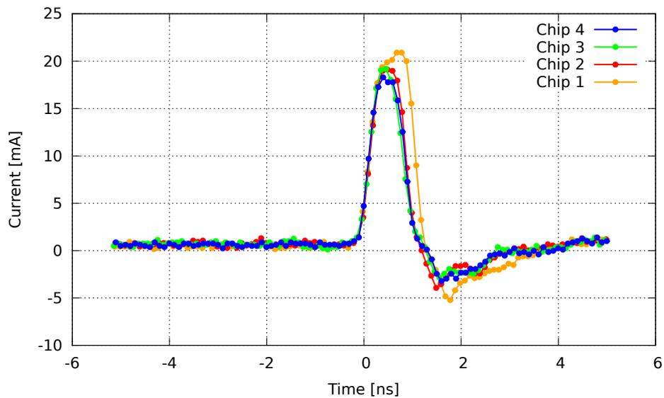
Figure 5.16: The electrical answers of the four driver ICs corresponding to the input signals in 5.15. The correlation is much better than for the LVDS signals. The y-axis shows the current corresponding to the voltage drop over a  $50\Omega$  resistor, measured with the DSO. The x-axis is the time in ns. Every point on the curves corresponds to one sample from the oscilloscope.
