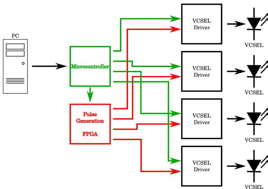
Figure 5.12: A block diagram for the circuitry of the prototype electronics of a QKD transmitter module. Short pulses are generated using a FPGA and are translated into modulation currents by four VCSEL drivers, each of which drives one VCSEL. In addition a microcontroller is used to set the bias and modulation currents of the drivers, as well as to control the FPGA.
