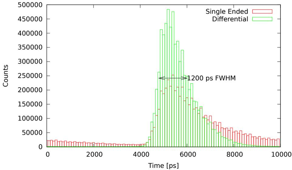
Figure 5.11: The arrival times for a single ended and a differentially connected VCSEL driven with the ONET8501V.
