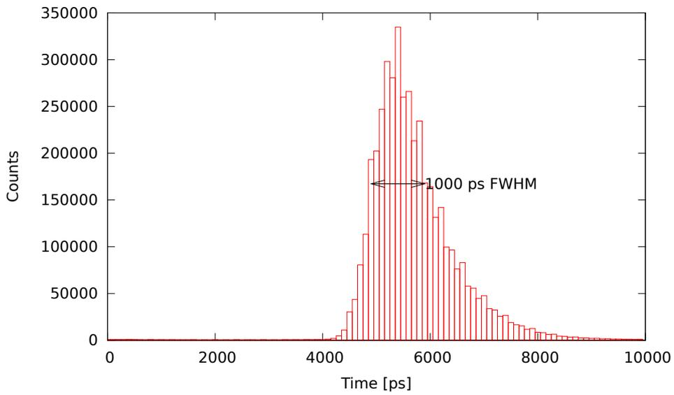
Figure 5.7: Arrival times for photons in a pulse produced with the ONET4291VA.
