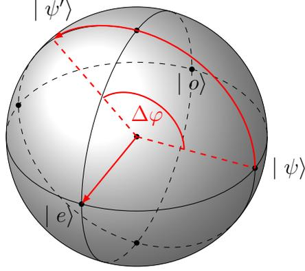
Figure 3.1: The influence of a birefringent medium on the state  $|\psi\rangle = 1/\sqrt{2}(|o\rangle + |e\rangle)$  on the Poincaré sphere. Any state will be rotated around the  $|e\rangle$ -axis by  $\Delta\varphi$ .
