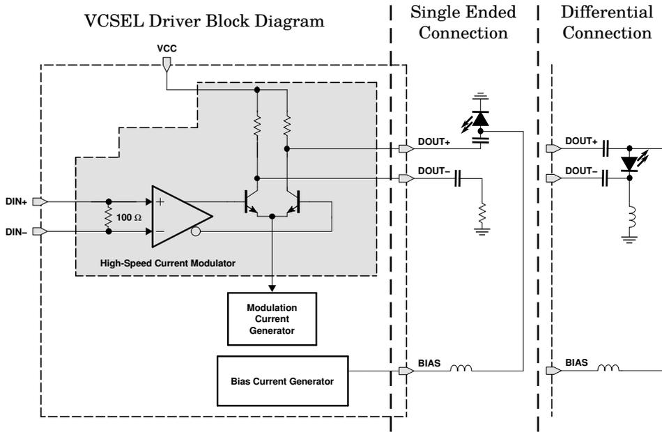
Figure 5.9: A simplified block diagram for the driver IC. The differential input signal  $DIN_{\pm}$  is interpreted by a comparator. The inverted and normal output of the comparator then each control a transistor, for turning the modulation current on or off. The difference of the external differential wiring, compared to the single ended wiring is shown on the left side of the scheme, where circuitry at the output side of the IC is shown again. Block diagram inferred from datasheet [40].
