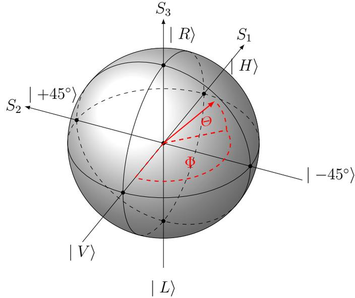
Figure 2.3: A polarization state represented as a vector on the Poincaré sphere, depicted in red and determined by the two angles  $\Phi$  and  $\Theta$ . The three Stokes parameters represent the projections on the principal axes of the sphere.
