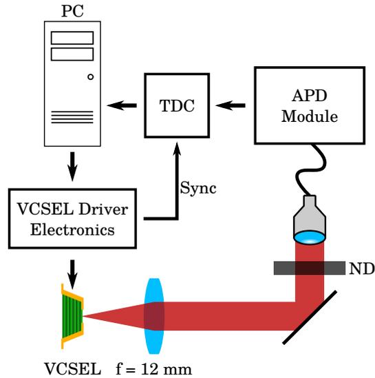
Figure 5.5: Setup used for determining the intensity contrast between the on and off state of the VCSELs. The VCSEL was driven with three different ICs and the resulting light pulses analyzed using an APD module and a TDC. The complete circuitry for driving the diode were controlled via a PC. The driving electronics and the TDC where synchronized via a 40 MHz reference signal.
