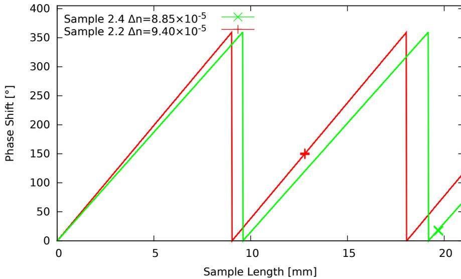
Figure 3.4: The phase shifts measured for both samples. The measured values for both samples are depicted with crosses, while the solid lines show the phase shift as a function of the sample length. These curves were fitted to the measured values to yield the values for the birefringence  $\Delta n$ .
