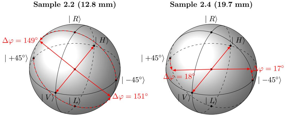
Figure 3.3: The red arrows represent the output polarizations on the Poincaré sphere, as measured with the polarimeter for both samples. The horizontal and vertical polarizations are not rotated, whereas the  $\pm 45^\circ$  polarizations are rotated with the phase shift indicated beneath the red arrows. The dashed arrows indicate the rotation direction.
