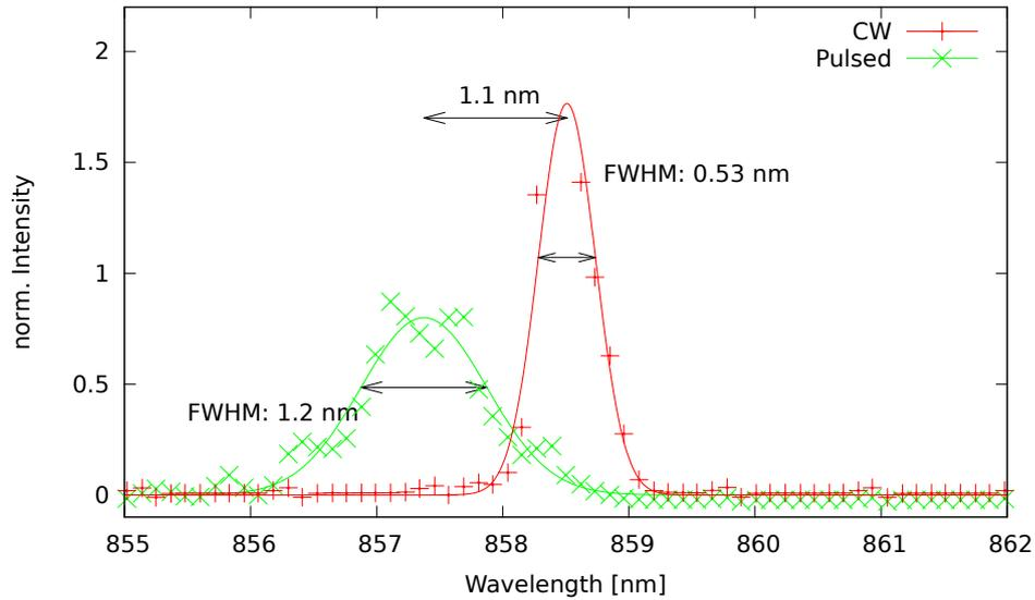
Figure 4.5: The spectrum of the same VCSEL as before also depicted in red, however, now driven in pulsed mode. The broadening of the spectrum is clearly visible.
