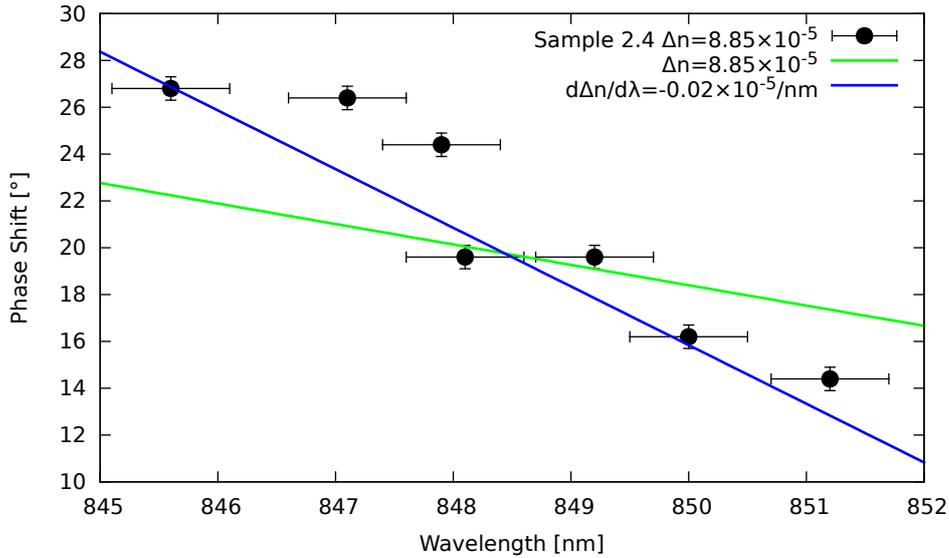
Figure 3.6: The rotation of the output polarization with respect to the central wavelength. The blue line shows the best fit with a constant dispersion for  $\Delta n$ . The green curves corresponds to the constant birefringence found in the previous section, where no dispersion  $\frac{d\Delta n}{d\lambda} = 0$  was assumed. The error bars depict the measuring inaccuracy of the used spectrometer and the polarimeter.
