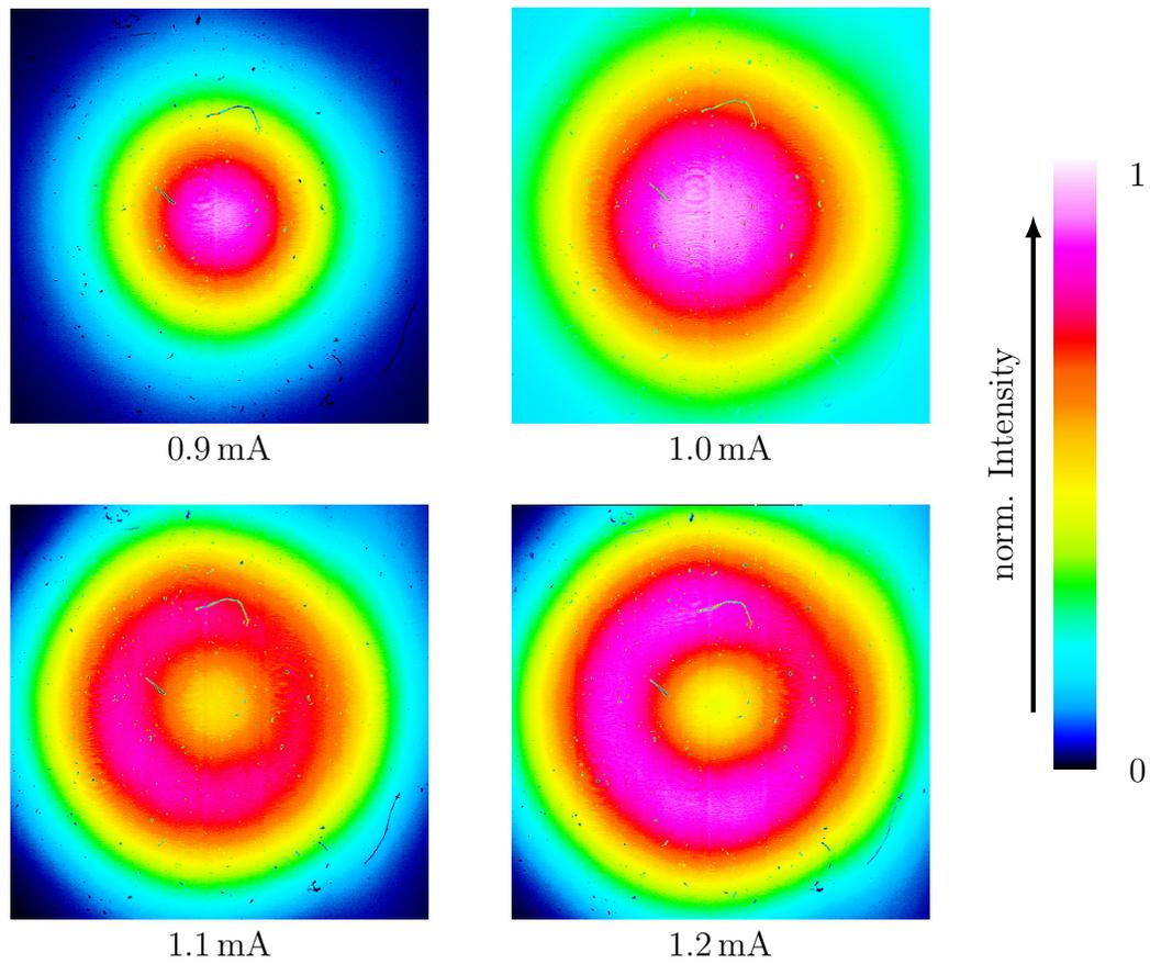
Figure 4.11: Four spatial modes emitted at different currents. The current increases from the top left to the bottom right picture. The intensity is color coded as indicated by the bar.
