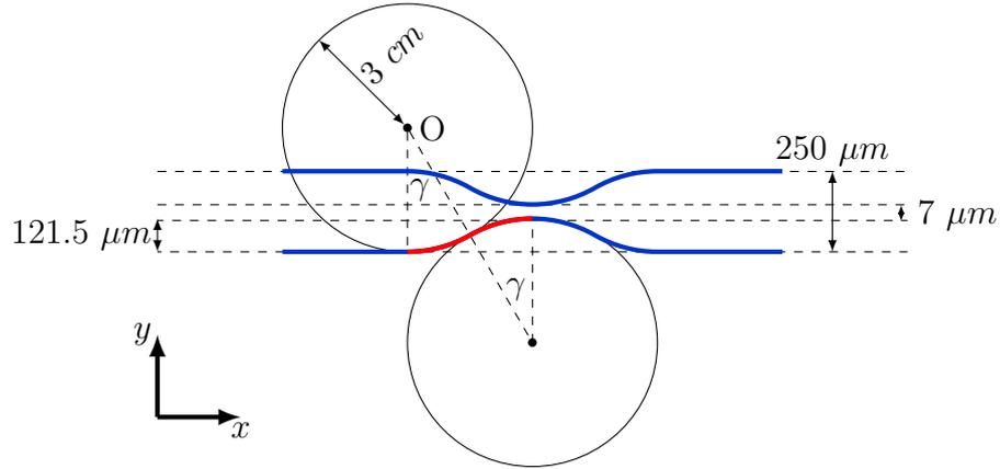
Figure 3.13: The length of the curved parts of the waveguides can be calculated from their geometry. The waveguides start with a distance of  $250 \mu\text{m}$  and come as close as  $7 \mu\text{m}$ . That means one combination of left and right curvature bridges a distance of  $121.5 \mu\text{m}$  in  $y$ -direction.
