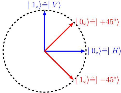
Figure 2.2: The four quantum states used for the BB84 protocol. The two mutually unbiased, orthogonal bases are depicted in blue and red, respectively. The vectors shown illustrate the states as polarizations of light. Each state confines an angle of  $45^\circ$  with his neighbor.
