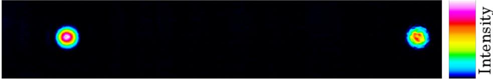
Figure 3.9: The two output modes of a directional coupler imaged with a linear camera. On the left side the output  $O_1$  is visible and on the right side the output  $O_2$ . The bar indicates the color coding of the intensity from 0 at the bottom to 1 at the top.
