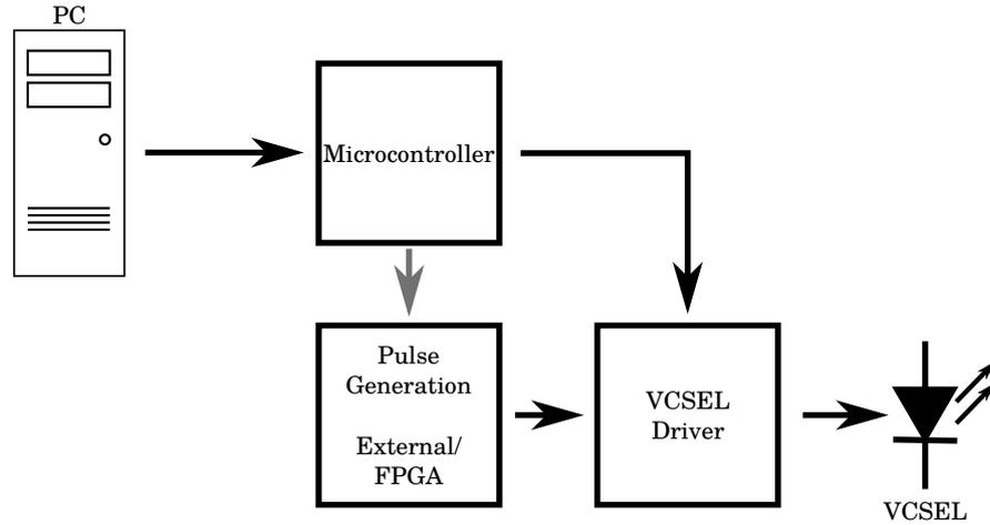
Figure 5.3: A sketch of the schematics of the evaluation boards. A microcontroller is used to control the bias and modulation currents, applied to the VCSEL via the driver ICs. The first evaluation board built for the LTC5100 used an external source for data input, whereas the second evaluation board, testing the ONET4291VA and ONET8501V, was equipped with and FPGA for generating short pulses.
