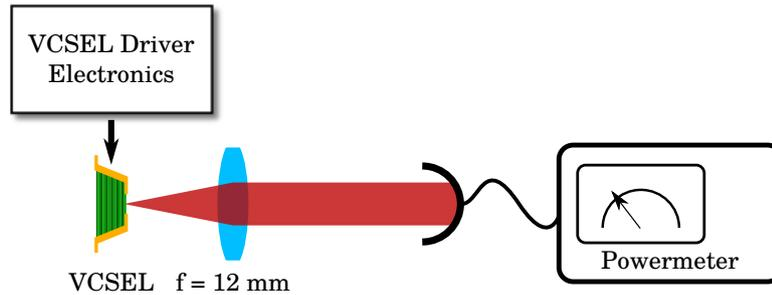
Figure 4.9: Setup for measuring the power-current curve. The light emitted by a VCSEL was collimated by an aspheric lens and then measured using a powermeter.
