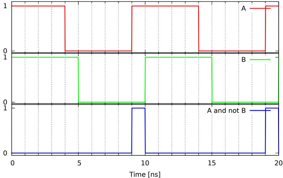
Figure 5.4: Principle of the short pulse generation on a FPGA. By shifting a clock signal with 50% duty cycle by 1 ns and then applying the logical operation  $A \wedge \neg B$ , short pulses with a width of 1 ns and a repetition rate of  $f_{rep} = 100$  MHz are created.
