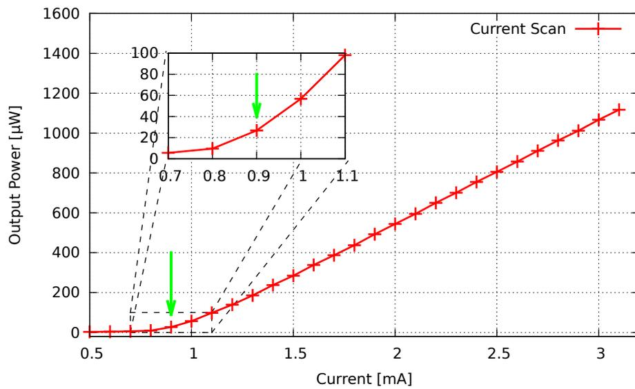
Figure 4.10: The output power of a VCSEL vs. the driving current. The green arrows mark the threshold current. The inset is a zoom into the region around the threshold.
