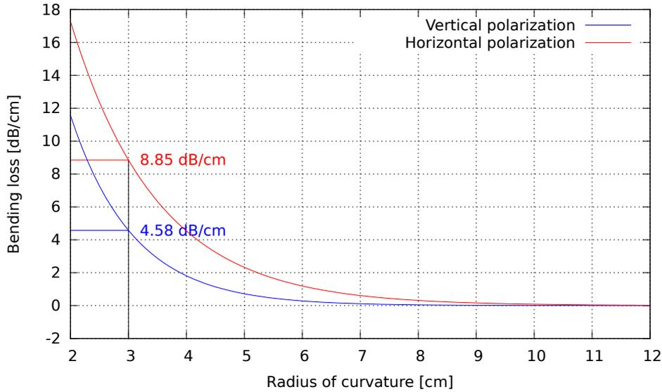
Figure 3.12: Bending losses in dB/cm for different bending radii and polarizations. The horizontal and vertical polarizations agree with the ordinary and extraordinary axes of the waveguide. The curves were supported by the group of Roberto Osellame.
