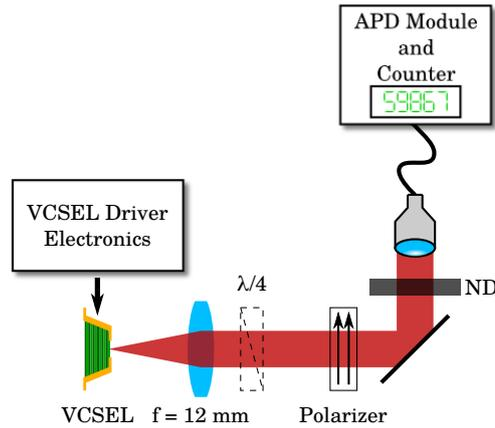
Figure 4.6: The setup used for measuring the DOP. The VCSEL can be operated either in pulsed or continuous mode. The light emitted is then collected by a lens and passes an optional  $\lambda/4$ -plate and a polarizer. The transmitted photons are counted using an APD module together with a counter. A neutral density filter (ND) was used to avoid saturation of the APD.
