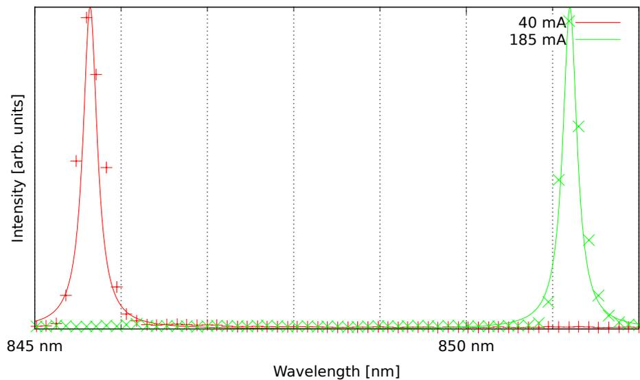
Figure 3.5: Two spectra of the narrow bandwidth laser used to measure the depolarization. An overall scanning range of approximately 6 nm was achieved. The points show the measured data from a spectrometer and the solid lines are fits to that data, with a fixed width of 0.2 nm. The resolution of the spectrometer is 0.13 nm/pixel.
