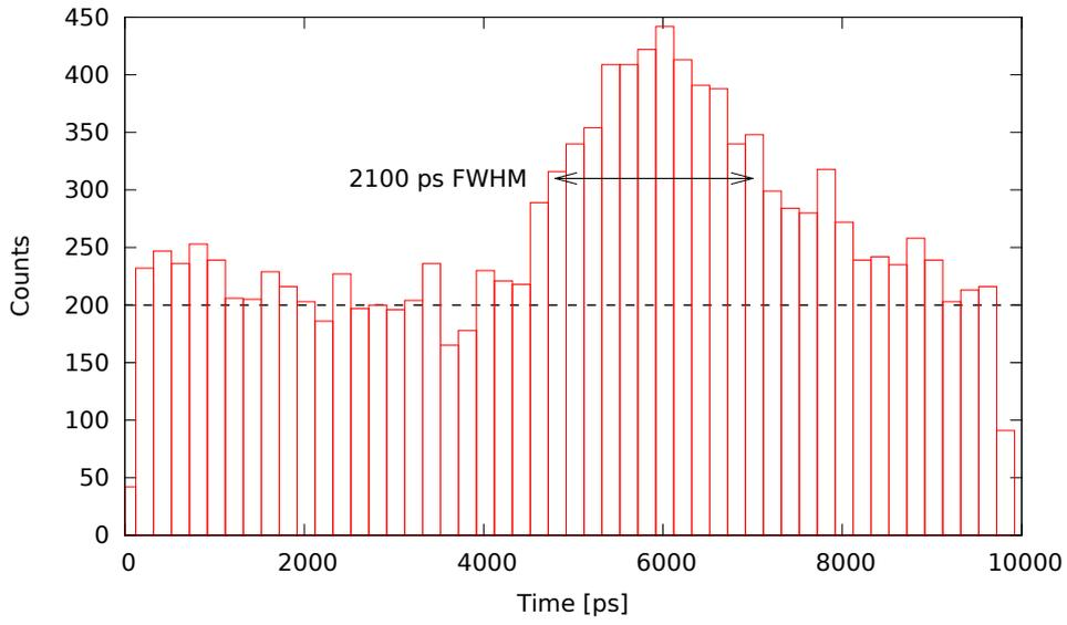
Figure 5.6: The arrival times of photons contained in the pulses produced, with the LTC5100 VCSEL driver.
