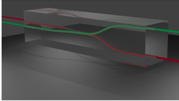
Figure 6.1: An alternative geometry for the integrated beamsplitters, where the possibility of a three dimensional path is used to exchange the bending between  $|V\rangle$  and  $|H\rangle$ . Both waveguides of the directional coupler start and approach each other in a horizontal plane. However they, after brought into close proximity, move away from each other in vertical direction, following a true three dimensional path.
