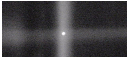
Figure 4.6: After aligning the MOT we observe a small cloud of cold rubidium atoms (the bright spot) and the fluorescence from the background gas in the cooling laser beams for a big magnetic field gradient with a CCD camera.
