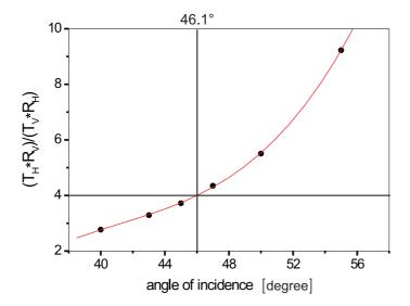
Figure 5.5: The decisive ratio for the setting of the adjustable beam splitter
