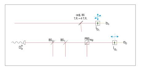
Figure 5.7: The adj.BS has to be mounted in  $b_0$ . It is aligned exactly to the right splitting ratio.
