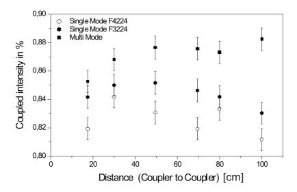
**Figure 5.2:** Dependence of the coupling efficiency for different single mode fibers (F3224, F4224) and a multi mode fiber (AS S50/125Y) the distance
