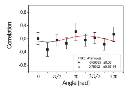
Figure 6.7: The correlation function for rotating a half wave-plate in a, with fixed basis  $x (+/-45^{\circ})$  in b conditioned on an outcome  $z_c = V$
