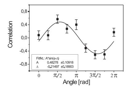
Figure 6.8: The correlation function for rotating a half wave-plate in a, with fixed basis x (+/-45°) in b conditioned on an outcome  $z_c=H$
