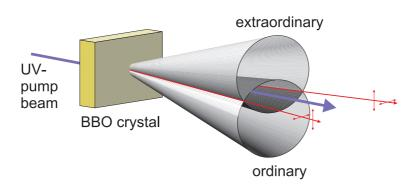
Figure 4.1: The emission cones of the degenerate type II down conversion emission
