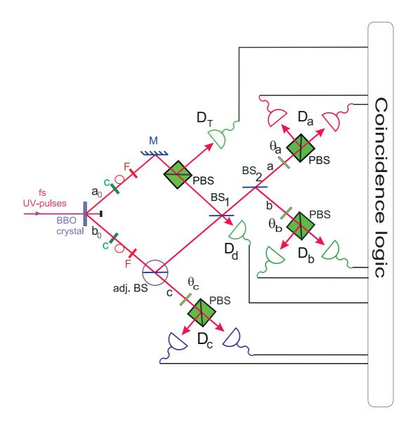
Figure 4.2: Experimental setup for the demonstration of the entangled three-photon W-state where C, F, M, BS, adj. BS and PBS stand for compensator cristal, filter, mirror, non-polarizing beam splitter, adjusting beam splitter with a reflection coefficient  $R_V = 2R_H$  and polarizing beam splitter. Three polarization analyzers with wave plates set to  $(\theta_i(i = a, b, c))$  are used.
