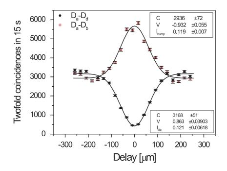
**Figure 5.11:** Coincidence dip  $(D_a^H, D_{dip}, \text{ full circles})$  and bump  $(D_a^H, D_b^H, \text{ open circles})$ . The maximum interference occurs at zero delay between the photons arriving at BS<sub>1</sub>. The risibilities are  $V_{dip} = 86.4 \pm 0.4$  and  $V_{bump} = 93.3 \pm 0.6$
