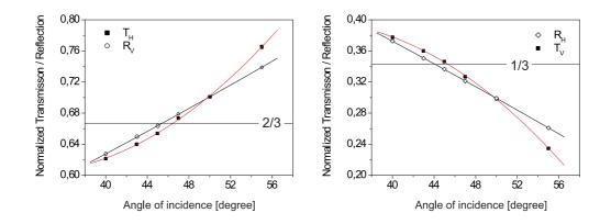
Figure 5.4: The dependence of the transmission and reflection coefficients on the angle of incidence
