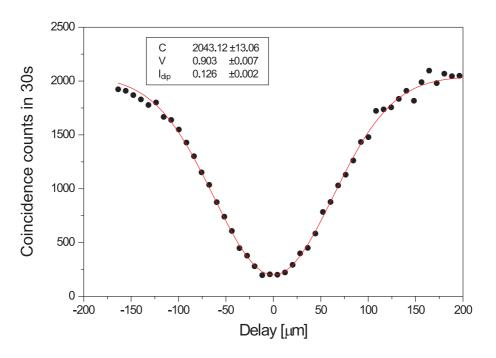
Figure 5.10: A HOM-dip measured with single mode fibers at the detectors for mode selection.
