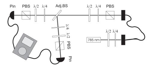
Figure 5.3: Setup to characterize the adj. beam splitter:
