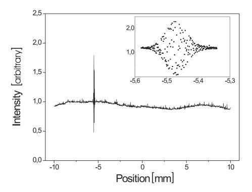
Figure 5.9: The scan for the position where the pulses overlap. The small picture shows a scan over the range where the overlap was expected. One can also see, that the coupling stays very stable over the whole range
