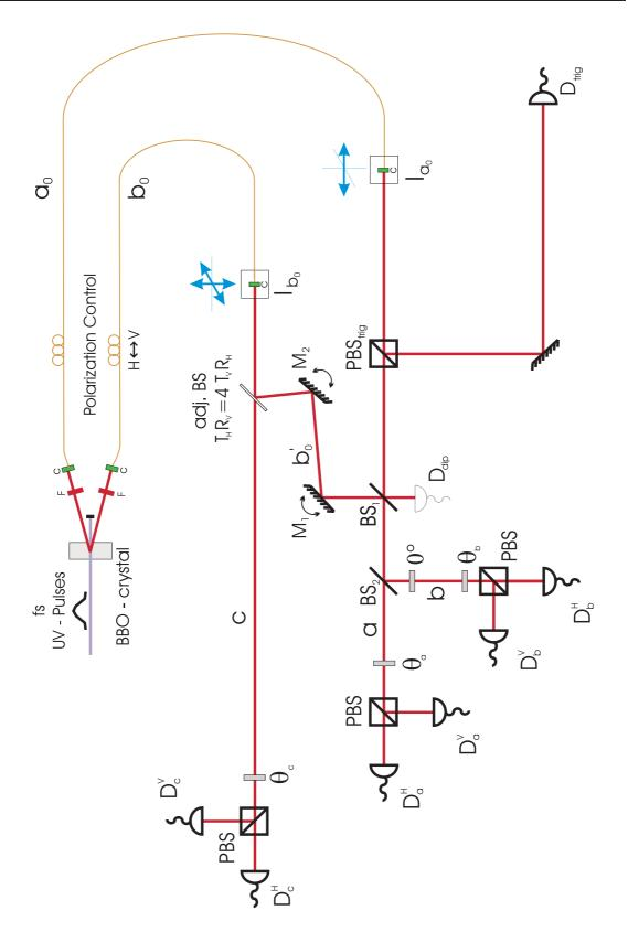
Figure 5.1: Overview of the experimental setup used for the preparation of the Three-Photon Entangled W-state
