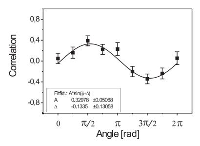
Figure 6.6: The correlation function for rotating a half wave-plate in a, with fixed bases x  $(+/-45^{\circ})$  in b and z (H/V) in c
