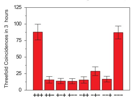
Figure 6.2: Three-fold coincidences in 3 hours of a xxx-measurement, i. e. with  $\lambda/2$  wave plates at 22.5°
