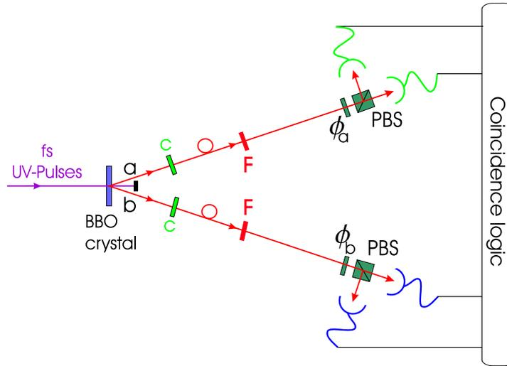
**Figure 1.** Experimental setup for the demonstration of two-photon entanglement where C, F, and PBS stand for fiber coupler, filter, and polarizing beam splitter respectively. The 2 photons are emitted into modes  $a$  and  $b$ . Two polarization analyzers with different settings ( $\phi_i (i = a, b)$ ) are used
