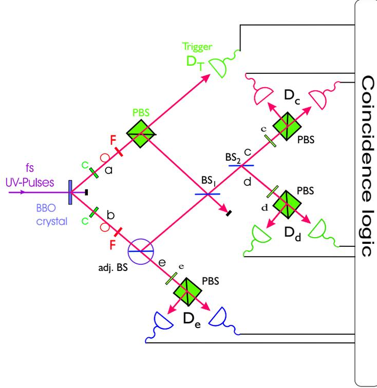
**Figure 3.** Experimental setup for the demonstration of three-photon entanglement W state where C, F, BS, adj. BS and PBS stand for fiber coupler, filter, non-polarizing beam splitter, adjusting beam splitter with a  $R_H = 2R_V$  reflection coefficient and polarizing beam splitter respectively. Three polarization analyzers with different settings ( $\theta_i (i = c, d, e)$ ) are used
