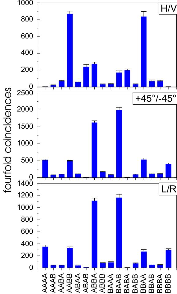
**Figure 4.** Fourfold coincidences in 16 hours of measurement, for the entangled 4-photon state (Eq. 7), with different polarization settings where A and B stand for (H, +45°, left) and (V, -45°, right) polarization respectively.
