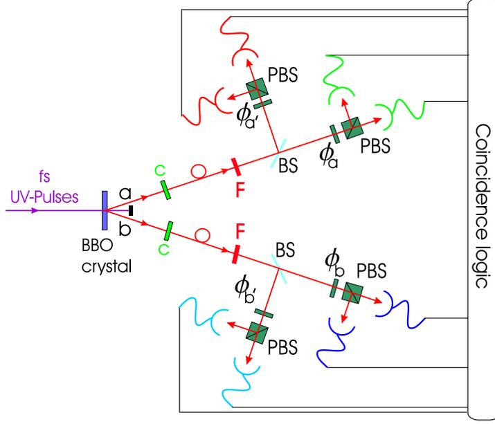
**Figure 2.** Experimental setup for the demonstration of four-photon entanglement where C, F, BS, and PBS stand for fiber coupler, filter, non-polarizing beam splitter and polarizing beam splitter respectively. The 4 photons emitted into modes a and b are split by BS. Four polarization analyzers with different settings ( $\phi_i (i = a, a', b, b')$ ) are used
