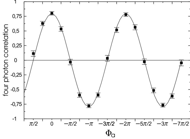
**Figure 5.** Quantum correlation function (Eq. 13) on the angle  $\phi_a$  and the other analyzers are fixed at angle  $\phi'_a = \phi_b = \phi'_b = 0$ . The data shows a visibility of  $V \simeq 79.3\%$ .
