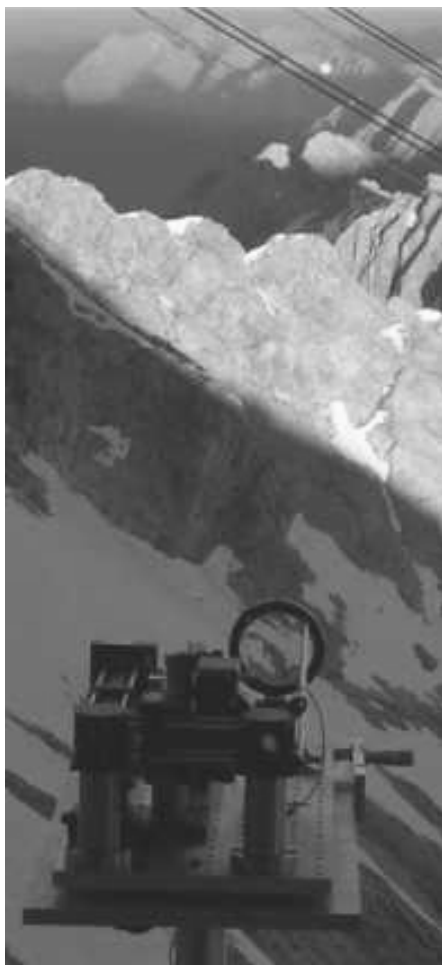
Figure 3 The Alice breadboard in the foreground with the green alignment laser clearly visible on Karwendelspitze in the background
