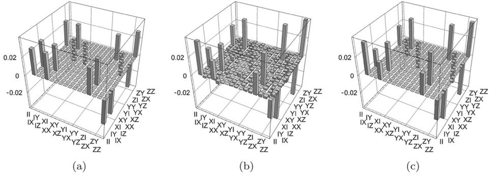
Fig. 2. (a)  $\chi$  matrix of the QPT for an ideal phase gate, (b) for the experimentally realized gate and (c) for a theoretical model fit to the experimental data. The imaginary part of the experimentally obtained  $\chi$  consists of noise only which is comparable to the one in the real part.
