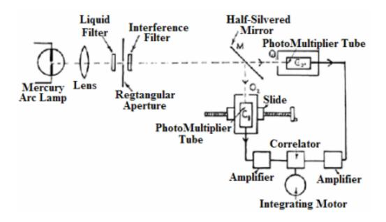
Figure 2.6: Schematic representation of the Hanbury Brown-Twiss (HBT) intensity correlation experiment. Q1 was placed on a translation stages, so that the two detectors could register light separated by a distance d. In this way the spatial coherence of the source could be investigate. (After R. Hanbury Brown and R. Q. Twiss [1].
