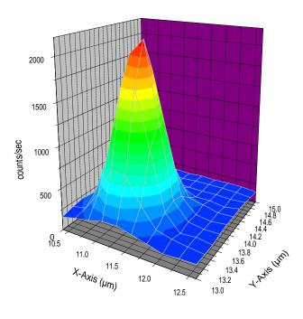
**Figure 5.5:** This fluorescence scan  $(2\mu m \times 2\mu m)$  of a IIa diamond sample performed with the same parameters as in figure 5.4 with SIL and we observed high intensity compared to figure by a factor of 6.
