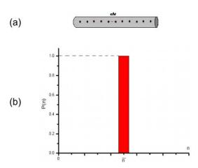
Figure 2.3: (a) Beam of light containing a stream of photons with a fixed-time spacing  $\Delta t$  between them. (b) Photon counting statistics for such a beam.
