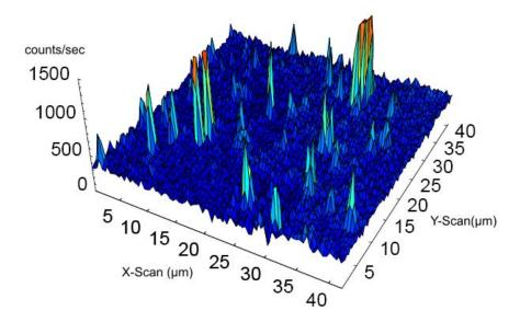
**Figure 5.8:** Scheme of the experimental measurements with images of single colour centers with SIL. Confocal fluorescence image  $(40\mu m \times 40\mu m)$  of SIV centers embedded in diamond with continuous-wave excitation at 685 nm.
