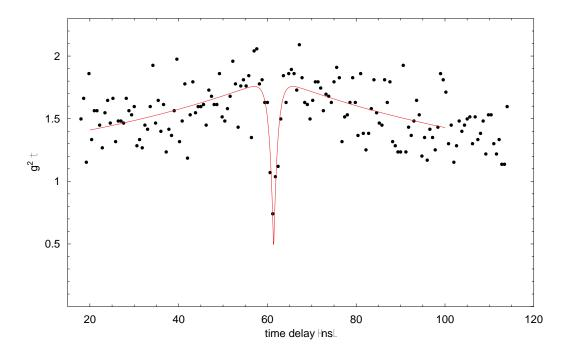
Figure 5.10: The fluorescence intensity autocorrelation function; the experimental data are shown in circle-shaped symbols, while the red line is the theoretical curve, calculated according to the procedure described in the text. The autocorrelation function shows a good contrast and presents a pronounced dip close to  $\tau = 60ns$ . Photon antibunching correlation measurements are carried out using the setup shown in figure 4.1.
