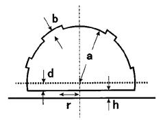
**Figure 5.11:** The schematic [59] of the typical errors in a hemisphere SIL: aspheric error **b**, a thickness error **d**, and an air gap **h**.
