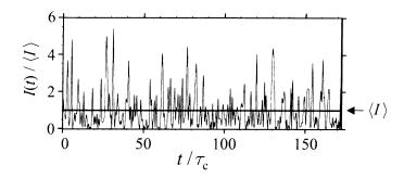
Figure 2.7: The computer generated time series (in units of the coherence time  $\tau_c$ ) for the cyle averaged intensity of Gaussian distributed light, assuming a light source with a Gaussian spectral profile [40].
