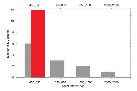
Figure 5.9: The histogram peak intensities for the SiV centers with and without SIL in  $40\mu m \times 40\mu m$  region of diamond sample. The number of SiV centers without SIL are indicated by the red bar. All the centers show the same count rate. The number of SiV centers with SIL are indicated by the gray bars. The SiV centers show different count rates with SIL.
