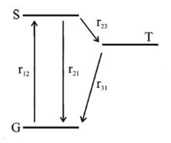
**Figure 5.1:** Schematic energy scheme *Jablonski Diagram* showing the ground (G), excited singlet (S), and triplet (T) states, and the various transition rates between the states [56].
