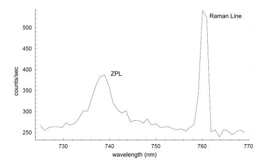
**Figure 5.3:** The narrow peak at 738 nm is the ZPL of the SiV centre The Raman scattering peak is at 760 nm.
