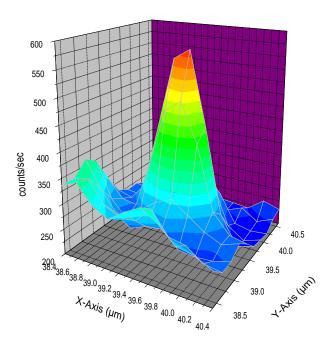
**Figure 5.4:** Fluorescence intensity raster scan  $(2\mu m \times 2\mu m)$  of a IIa diamond sample performed about  $2\mu m$  below the diamond surface showing luminescence from an isolated color center. The size of a pixel is 100 nm. The integration time per pixel is 1000 ms. One APD output in the HBT setup gives maximum counting rate 600 counts/sec.
