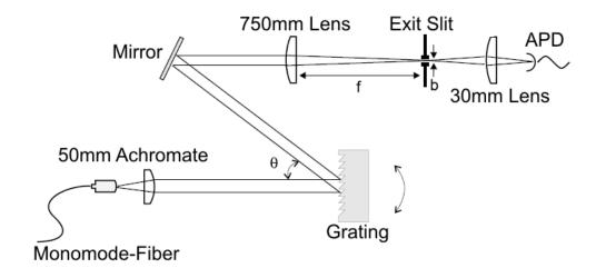
Figure 4.2: Schematic diagram of the home-made spectrometer.
