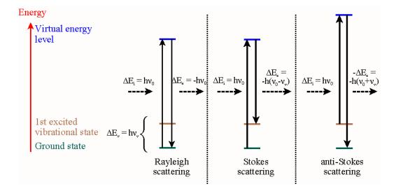
Figure 3.3: The different possibilities of visual light scattering: Rayleigh scattering (no Raman effect), Stokes scattering (molecule absorbs energy) and anti-Stokes scattering (molecule loses energy)
