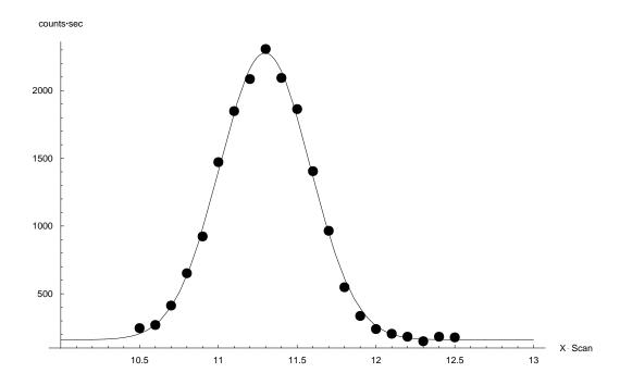
Figure 5.7: Line scan with SIL for figure 5.5 with  $0.5\mu m$  FWHM. It can be seen that the spot size becomes smaller compared to the case without SIL which explains the better resolution. The data is shown together with a gaussian fit, which is used to evaluate the signal and background levels. The signal (S) to background (B) ratio is S/B = 15.3 which is improved by using SIL.
