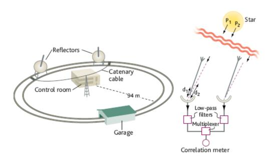
Figure 2.5: Coherence in light and matter; (Left) Sketch of the intensity interferometer used by Hanbury Brown and Twiss to measure the fluctuations in light from stars to deduce stellar sizes. (Right) Schematic of the Hanbury Brown and Twiss measurement of the correlations observed at two points from an extended optical source such as a star [39].
