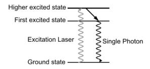
**Figure 1.2:** Typical optical excitation scheme for a single-photon source. A single quantum system is raised from its ground state to a higher excited state by a laser pulse, relaxes nonradiatively to a lower excited state, and emits a photon through spontaneous emission
