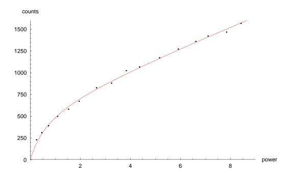
**Figure 5.2:** The fluorescence intensity saturation curve; symbols represent the experimental data and the red line a fit to data, according to equation (5.2) in the text.
