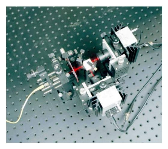
**Figure 4.3:** Hanbury-Brown-Twiss configuration for measuring the photon statistics.
