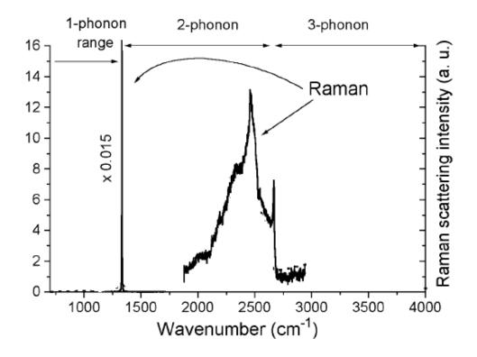
Figure 3.4: Room-temperature Raman spectra from IIa diamond
