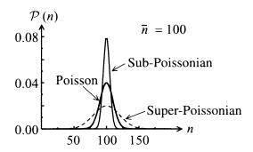
**Figure 2.2:** Comparison of the photon statistics for light. The distributions have been drawn with the same mean photon number.
