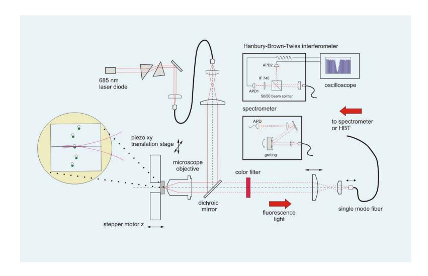
Figure 4.1: Schematic diagram of the SetUp.
