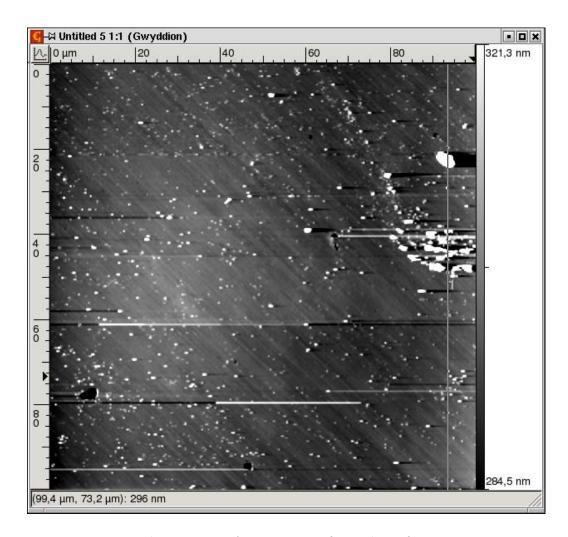
Figure 5.14: AFM picture of sample surface.
