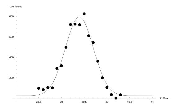
**Figure 5.6:** Line scan without SIL for figure 5.4 with  $0.6\mu m$  FWHM. The data is shown together with a gaussian fit, which is used to evaluate the signal and background levels. The line scan in figure shows that the signal (S) to background (B) ratio is S/B=4.
