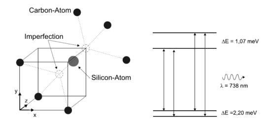
Figure 3.2: Theoretical model of energy scheme of SiV center [47].
