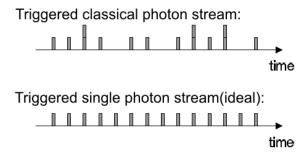
**Figure 1.1:** A pulsed classical source (top), and a pulsed single-photon source (bottom)
