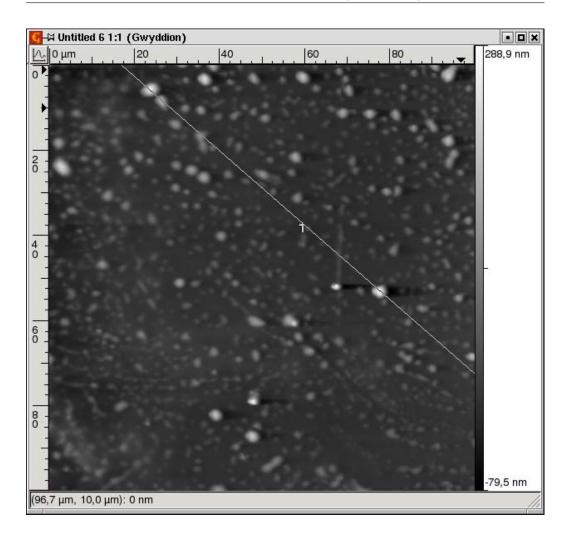
Figure 5.12: AFM picture of flatside of SIL.
