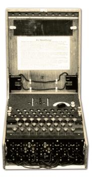
Figure 2.7: A picture of the Enigma encrypting/decrypting machine. This particular military model worked with three rotors.
